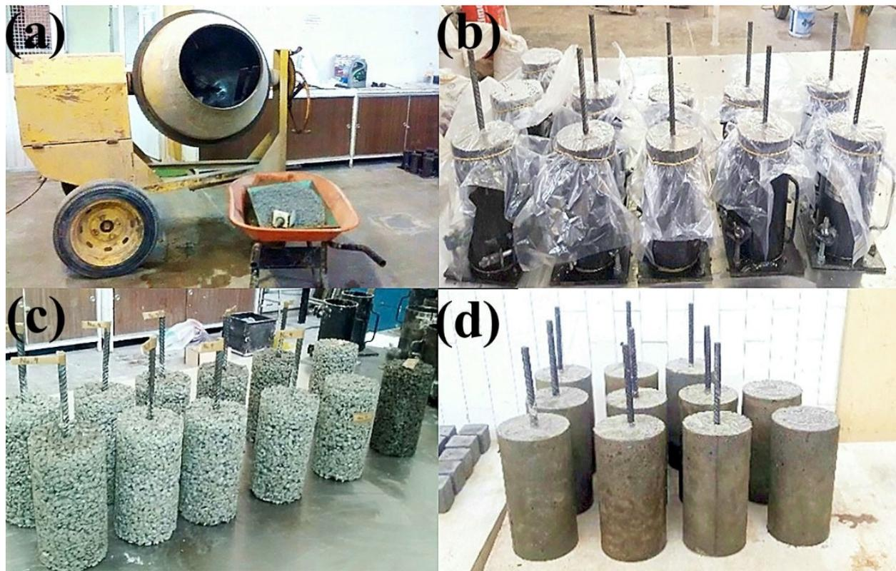
**Figure 3.** (a) Concrete mixer, (b) concrete cylinder specimens during setting, and (c) pervious and (d) conventional concrete specimens after curing for 28 days.
