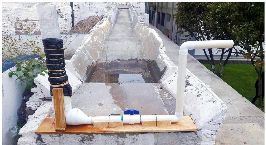
**Figure 4.** Variable-load permeameter.
