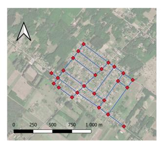
Figure 6. Base network topology. Red squares are the connection nodes.
