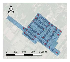
**Figure 9.** Manual determination of the nodes' range of influence. Red squares are the connection nodes, blue triangles are the consumption points.
