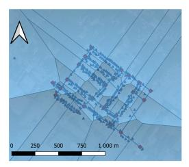
**Figure 10.** Determination of the nodes' range of influence based on Thiessen polygons. Red squares are the connection nodes, blue triangles are the consumption points.
