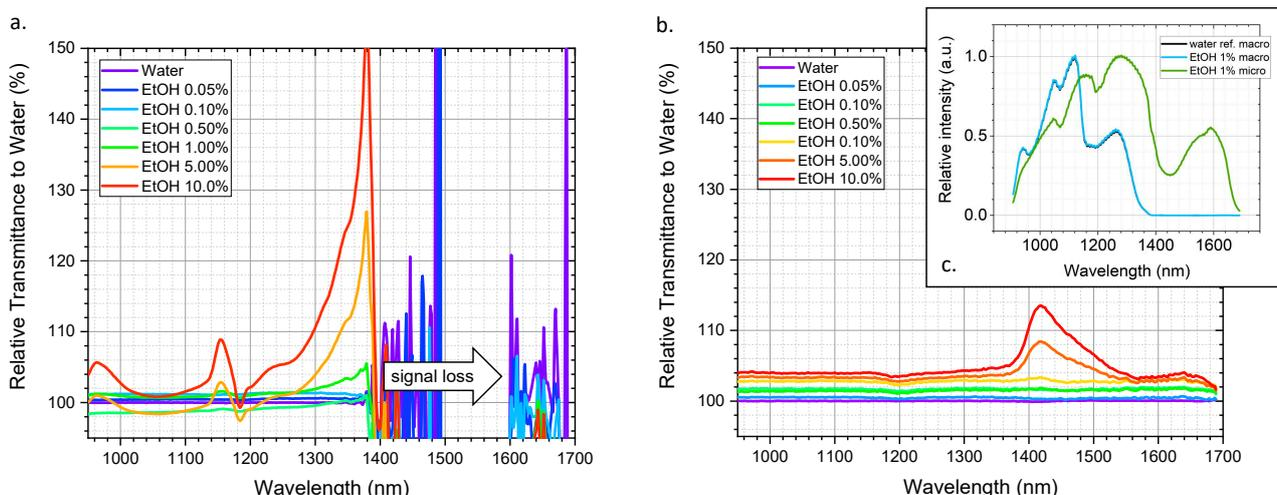
**Figure 1.** Concentration-dependent near-IR transmittance spectra for ethanol solutions (0.05, 0.1, 0.5, 1.0, 5.0, 10% *v/v*) compared to water as a reference in macroscopic (a) and microfluidic (b) HE (100  $\mu\text{m}$ , transmittance) cuvettes. Relative intensities (c) demonstrate a signal loss over a wavelength of 1400 nm.
