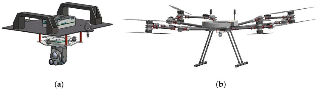
**Figure 18.** DragonEye 2: (a) dedicated custom payload case; (b) co-axial quadcopter configuration with the payload attached.
