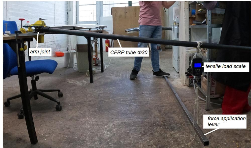
Figure 23. Physical testing of the aluminum joint.
