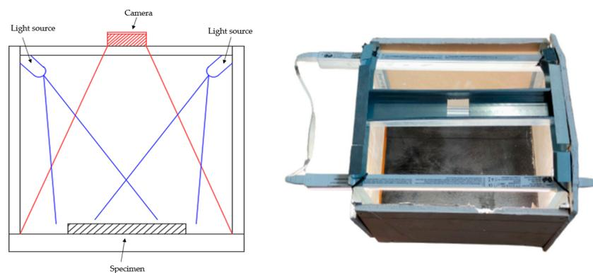
**Figure 5.** Laboratory equipment for taking photographs.
