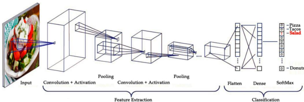
**Figure 2.** A simple CNN architecture [33].
