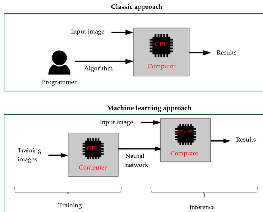
**Figure 1.** Schematic illustration of the classic approach where the algorithm is designed manually and the machine learning approach where a training set of labeled images is required [15].
