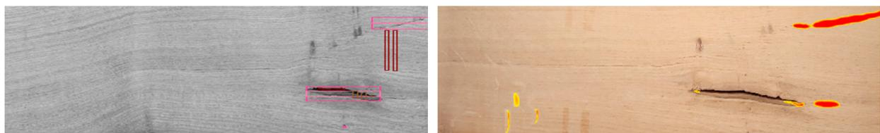
**Figure 10.** Defect detection on specimen 8 (**left**—software 1 image; **right**—software 2 image).
