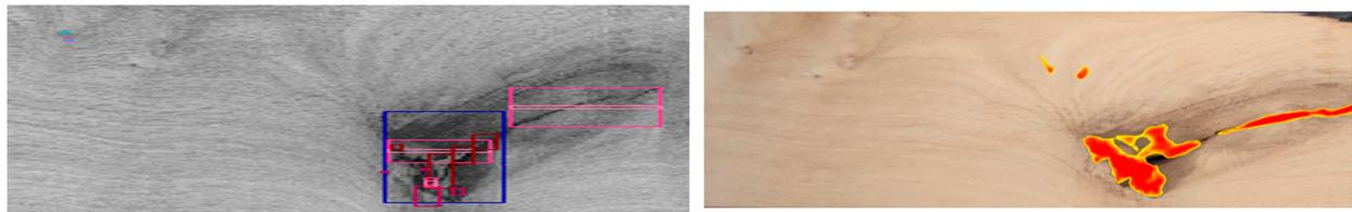
**Figure 8.** Defect detection on specimen 38 (**left**—software 1 image; **right**—software 2 image).
