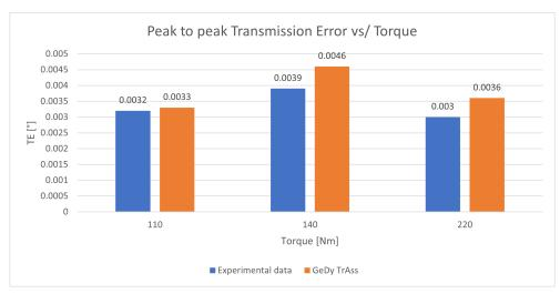
Figure 7. Comparison between measured and calculated PPTE.
