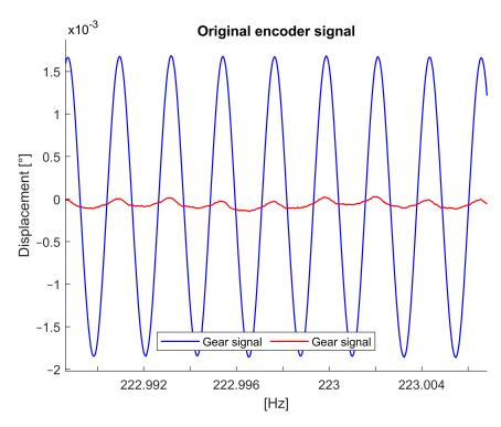
Figure 14. Synchronous angular displacement signals between two gears.
