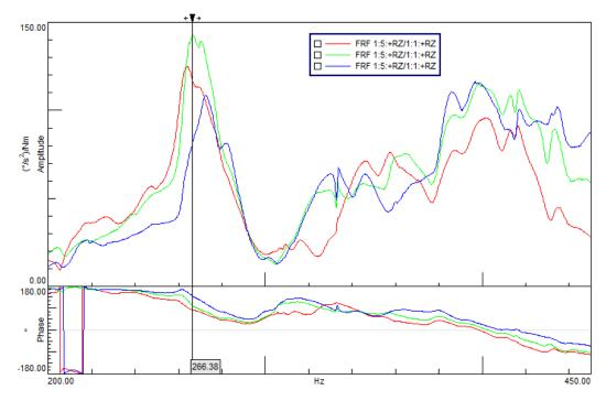
Figure 18. Example of a frequency shift for the single-contact pair around the meshing resonance.
