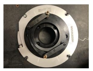
per revolution. Owing to the EnDat 2.2 interface, it is possible to obtain 536,870,912 (29 bits) position values per revolution.
