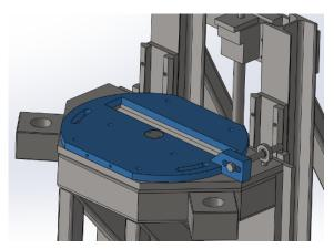
Figure 2. Plate for rotational micro-adjustments.
