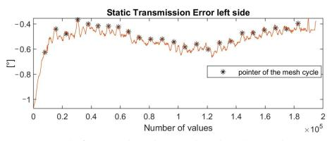
Figure 6. Example of an acquired STE; the stars indicate the tooth engaged.
