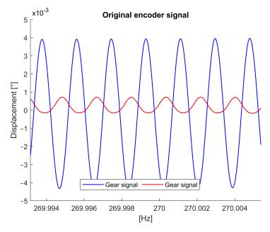
(a) Single-contact position resonance at 270 Hz with 90 Nm torque **Figure 15.** *Cont.*
