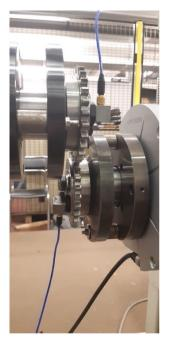
Figure 9. Triaxial accelerometers applied on the gears.
