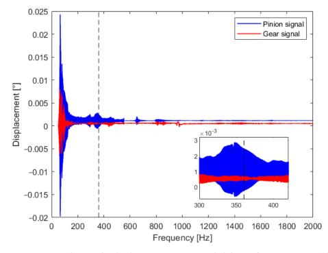
**Figure 13.** Encoder angular displacement output recorded during frequency sweep (the same as Figure 12).
