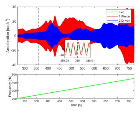
Figure 12. Frequency sweep and acceleration output recorded by accelerometers.
