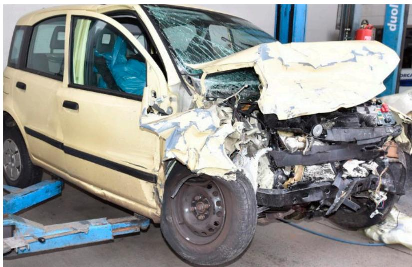
**Figure 17.** Frontal deformation image of a Fiat Panda of the same class in the EES catalog.
