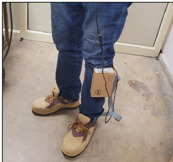
**Figure 7.** Volunteer wearing insole (inside shoe) and microcontroller using a Velcro strap during the qualitative and quantitative trials.
