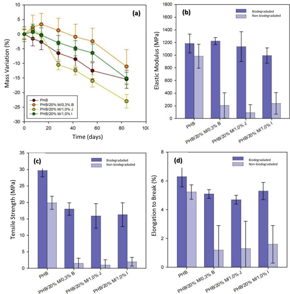
**Figure 9.** Results of the properties of PHB/babassu composites: (a) biodegradation results; (b) effect of biodegradation on the elastic modulus of the composites; (c) effect of biodegradation on the tensile strength of the composites; (d) effect of biodegradation on the elongation to break of the composites. Adapted with permission from ref. [198]. Licensed under CC BY-NC-ND 4.0.
