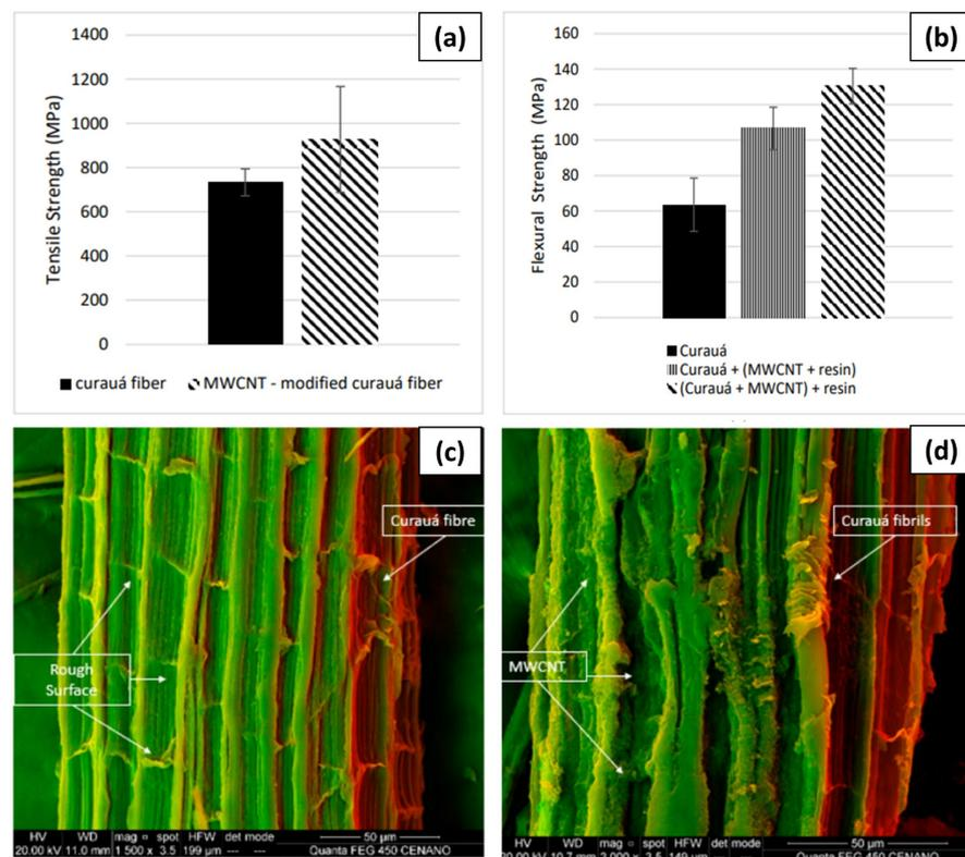
**Figure 14.** Results of epoxy matrix composites reinforced with curauá fibers and functionalized with MWCNTs: (a) tensile test results of the fibers; (b) flexural test results of the composites; (c) SEM micrograph of the “in natura” fiber; (d) SEM micrograph of the fiber functionalized with MWCNTs. Adapted with permission from ref. [249]. Copyright 2023, MDPI AG. Licensed under CC BY 4.0.
