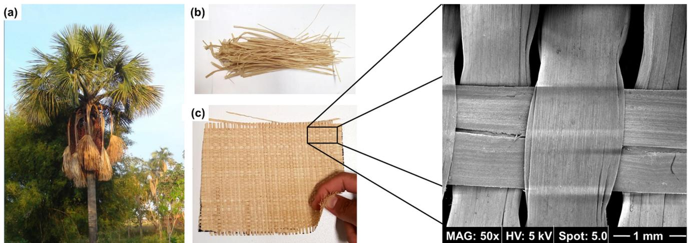
**Figure 10.** *Buriti (Mauritia flexuosa)*: (a) palm tree; (b) bundle of fibers extracted from the leaf; (c) fabric produced from the extracted fibers with an inset for viewing the weave from an SEM micrograph. Reprinted with permission from ref. [202]. Copyright 2020, Elsevier. Licensed under CC BY-NC-ND 4.0.
