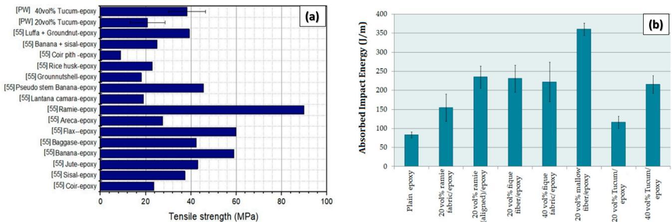
**Figure 21.** Results of the epoxy/tucum composites: (a) comparison of the tensile strength results of the epoxy/tucum composite with the literature; (b) comparison of the Izod impact resistance results. Adapted from ref. [286]. Copyright 2020, MDPI AG. Licensed under CC BY 4.0.
