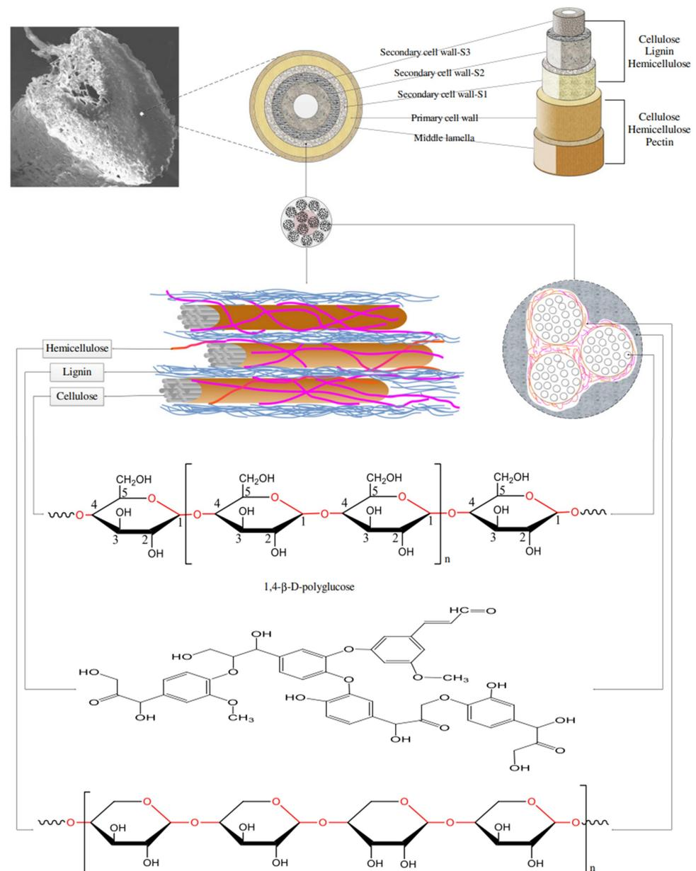
**Figure 3.** Schematic diagram of the natural fiber cell wall and its molecular structure. Reprinted with permission of ref. [68]. Copyright 2022, Elsevier.
