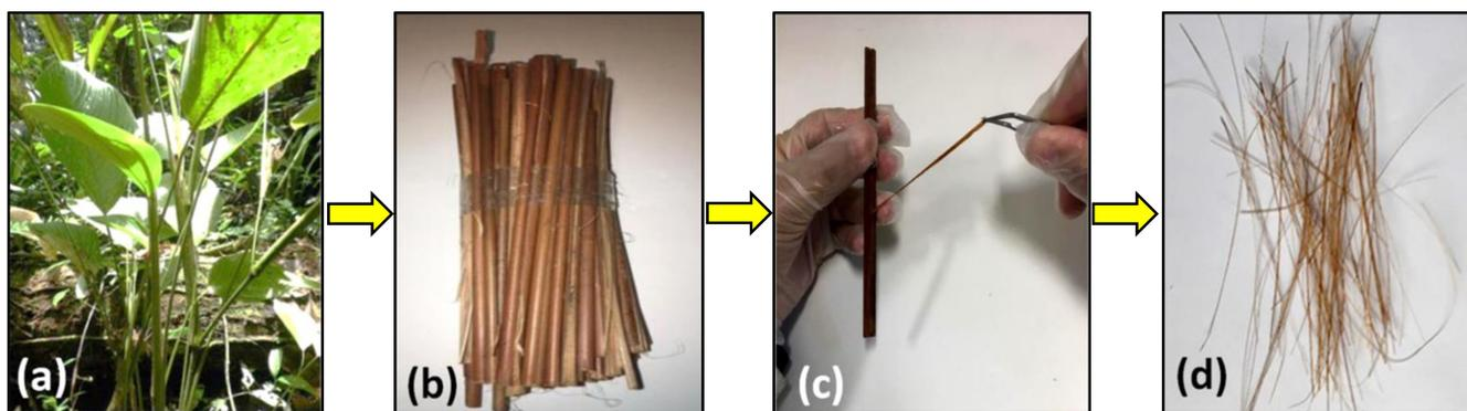
**Figure 15.** Guaruman (*Ischnosiphon Koern*): (a) guaruman plant; (b) as-received, mechanically divided splints from the stalk; (c) manual separation of fibers from the splint; (d) bunch of the final isolated fibers (d). Adapted with permission from ref. [253]. Copyright 2020, Elsevier. Licensed under CC BY-NC-ND 4.0.
