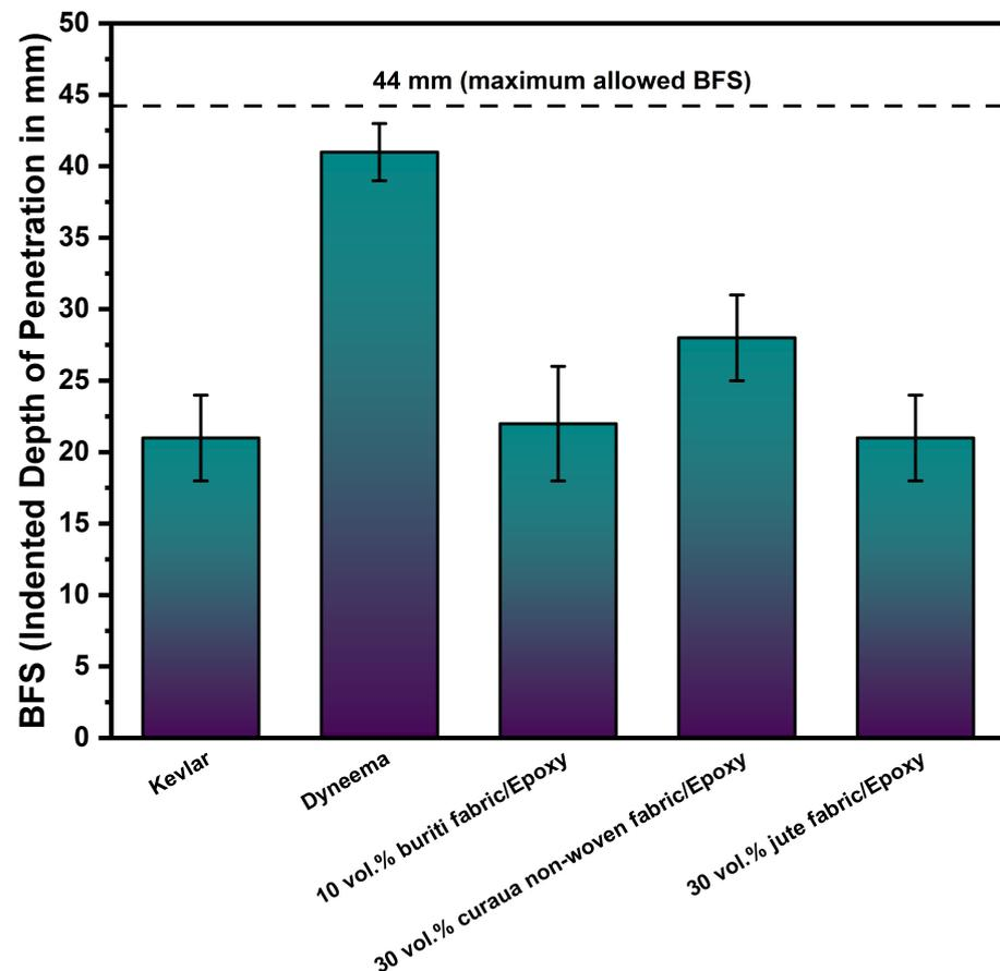
**Figure 11.** Comparison between the ballistic performance of both synthetic fabrics and natural fiber-reinforced polymer composites as the MAS second layer with the same thickness. Adapted from ref. [208].
