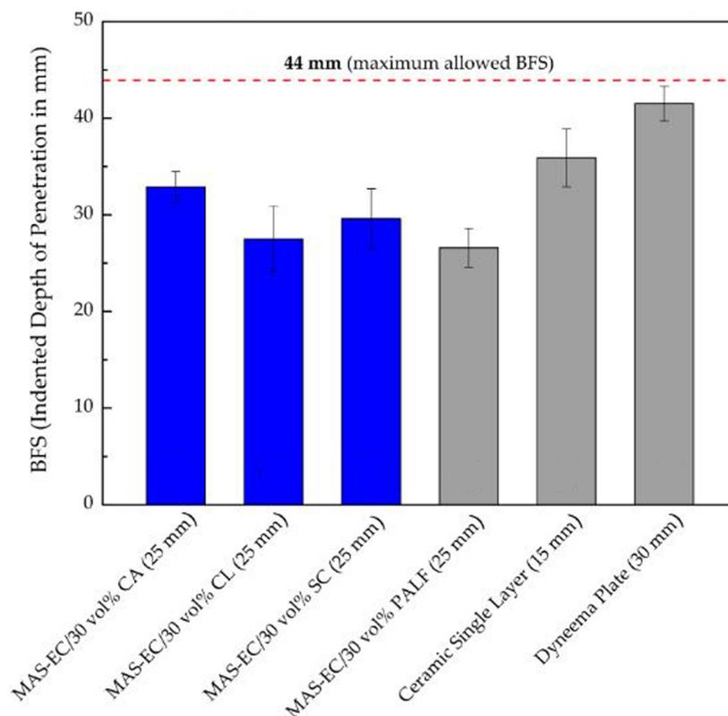
**Figure 16.** Results of BFS of composites produced with guaruman fibers after ballistic testing using  $7.62 \times 51$  mm ammunition. Reprinted with permission from ref. [254]. Copyright 2021, MDPI AG. Licensed under CC BY 4.0.
