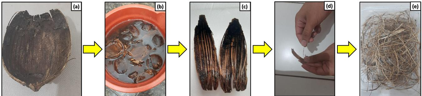
**Figure 8.** Steps of babassu fiber extraction: (a) babassu coconut in drying process for 48 h; (b) washing babassu; (c) babassu after washing, ready for defibrillation; (d) manual defibrillation process; (e) extracted babassu fibers. Reprinted with permission from ref. [193]. Licensed under CC BY-NC-ND 4.0.
