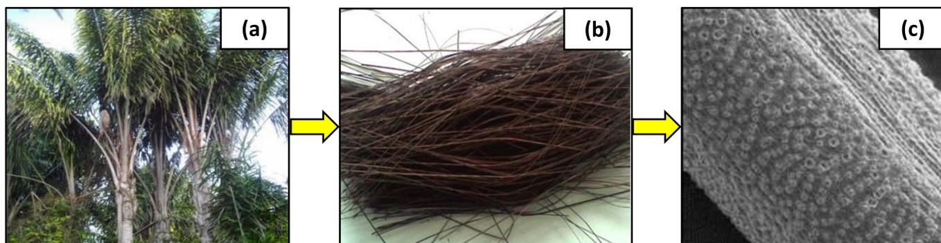
**Figure 18.** Piassava (*Attalea funifera*): (a) piassava palm tree; (b) piassava fibers extracted from leaf; (c) SEM micrograph of piassava fiber surface. Adapted with permission from ref. [261]. Copyright 2018, Scielo. Licensed under CC BY 4.0.
