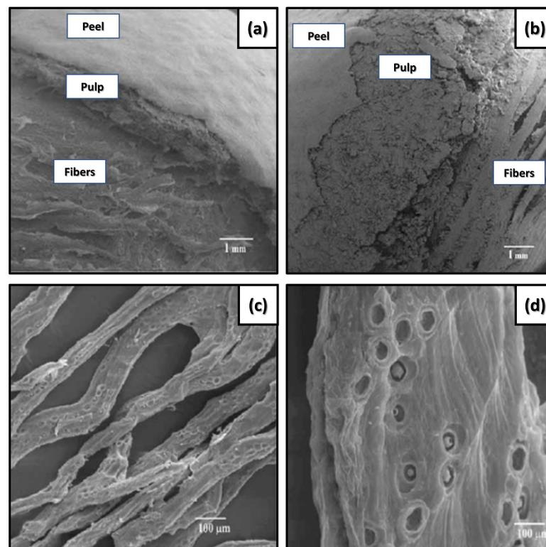
**Figure 6.** SEM micrographs of different regions of açai: (a) fruit micrograph indicating the regions of peel, pulp, and fibers; (b) another region indicating the position of peel, pulp, and fibers; (c) micrograph of fine açai fibers; (d) micrograph of a wider açai fiber, showing the presence of pores and imperfections on the surface. Adapted with permission from ref. [180]. Licensed under CC BY 4.0.
