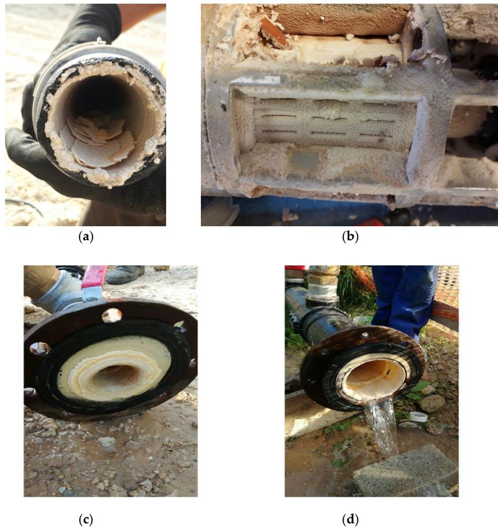
**Figure 2.** Deposition of limescale at the Sumayil North Site, Tel Aviv. (a) Suction pipe section between the well pump and the collector pipe. (b) Water intake opening in the well pump engine. (c) Pipe connection flange. (d) Pipe connection flange to the collector manifold.
