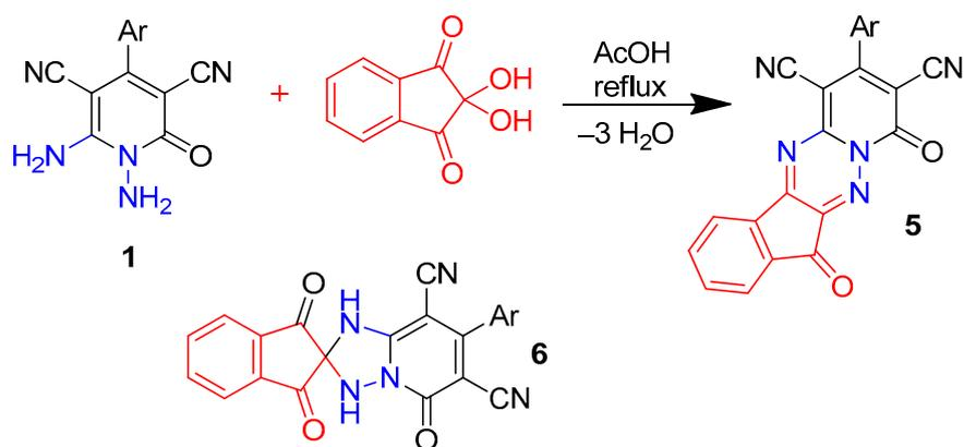
**Scheme 2.** The preparation of dihydroindeno[1,2-*e*]pyrido[1,2-*b*][1,2,4]triazines **5**.
