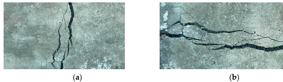
Figure 2. Cracking of 2% PPGF-ECC composite: (a) Slab 1; (b) Slab 2.
