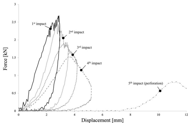
**Figure 3.** Force–displacement curves for the repeated low-velocity impacts.
