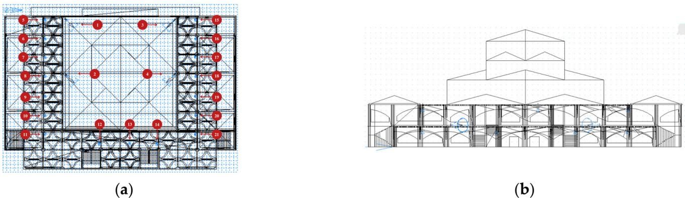
**Figure 5.** (a) The position of the 21 loudspeakers is indicated by the number inside the circle; (b) side view of the speaker position marked in blue.
