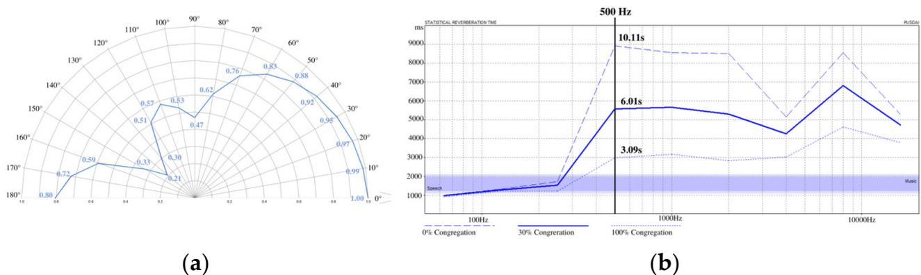
**Figure 6.** (a) Loudspeaker sound distribution pattern; (b) reverberation time chart.
