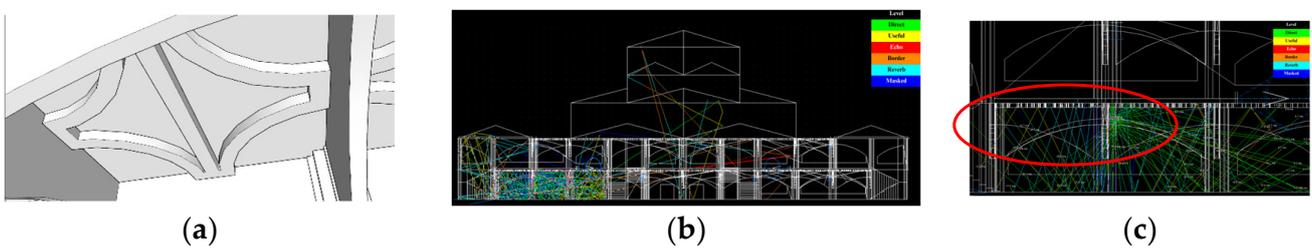
**Figure 8.** (a) Corridor ceiling design; (b) sound spread of loudspeaker 11 in the corridor; (c) speaker 11 sound spread due to ceiling design.
