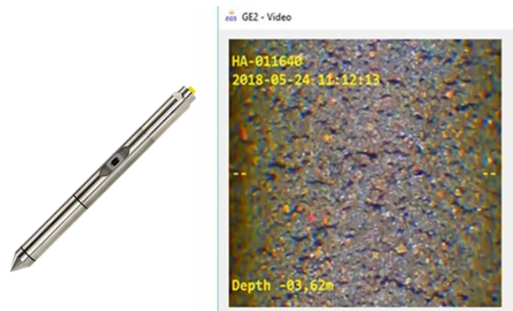
Figure 5. CPT video cone ( left ) and example of a video frame recorded from this module ( right ).
