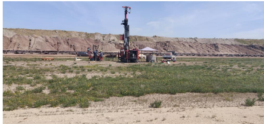
Figure 2. Royal Eijkelpkamp® sonic rig set-up on the mining waste dump in the Leipzig Coal Basin.
