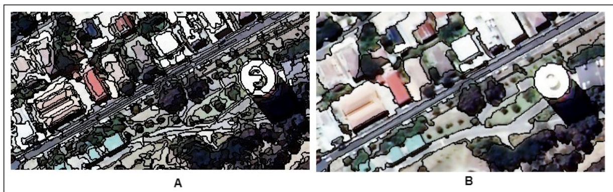
Figure 7. Subsets of segmentation results of a large parking lot and some roads from the satellite imagery. (A) shows over- and under-segmentation results at scale parameter 90, and (B) optimal segmentation results at scale parameter 110.
