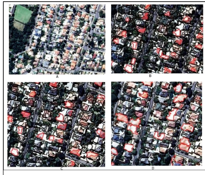
Figure 10. Subsets of image segmentation results performed with scale parameters of 40, 50, and 70 on the aerial photograph. Figure (A) shows the original scene; (B) shows the over-segmentation of building units at scale parameter 40; (C) shows the over- and under-segmentation of building units at scale parameter 50; and (D) shows the improved segmentation of building units at scale parameter 70.
