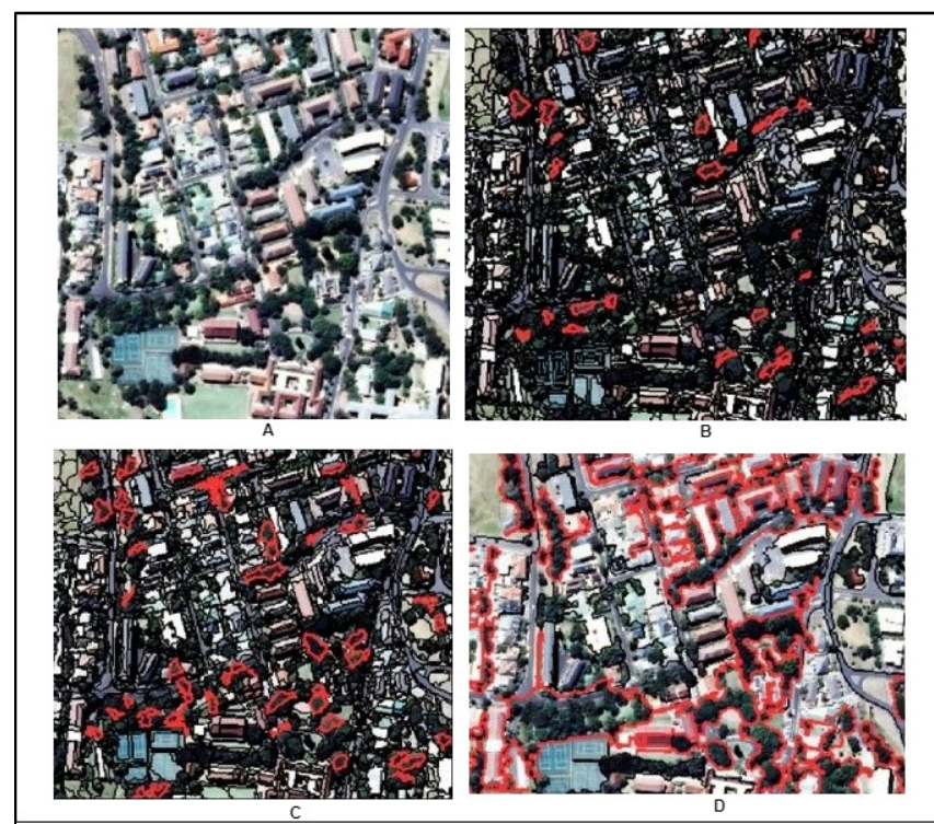
Figure 12. Subsets of segmentation results performed on the aerial photograph and showing urban trees segmented with scale parameters of 120, 130, and 150. Figure (A) shows the original scene; (B) and (C) show over-segmentation results of urban vegetation at scale parameters 120 and 130, respectively; and (D) shows optimal segmentation of urban vegetation at scale parameter 150.
