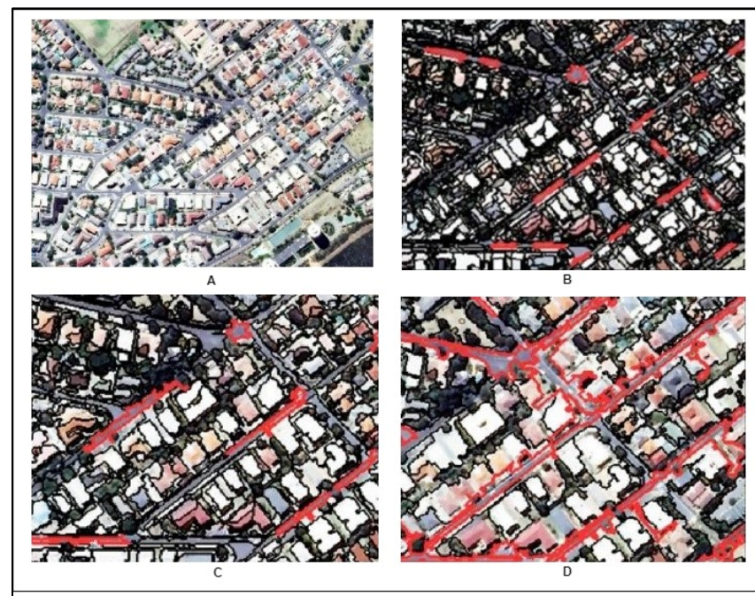
Figure 11. Subsets of segmentation results performed on the aerial photograph and showing urban roads segmented with scale parameters 90, 100, and 110. In (A), the figure shows the original scene; (B) and (C) show the over-segmentation of roads at scale parameters 90 and 100, respectively; and (D) shows an optimal segmentation of roads at scale parameter 110.
