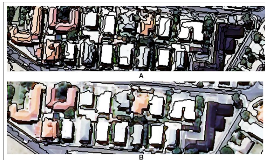
Figure 6. Subsets of regular and large building segmentation results from the satellite imagery. (A) over-segmentation results at scale parameter 50, and (B) optimal segmentation results at scale parameter 70.
