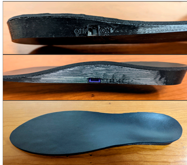
Figure 1. Insoles that currently use NCPF as a dynamic load sensor.
