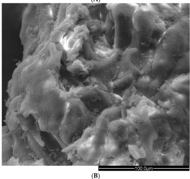
**Figure 3.** (A) Olive pit powder granule at  $600 \times$  magnification. (B) Olive pit powder granule at  $300 \times$  magnification.
