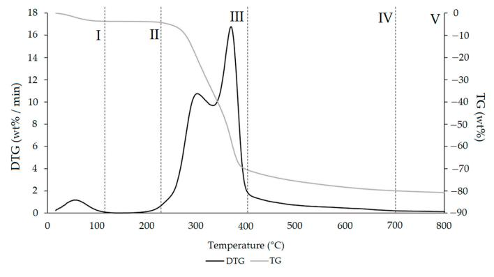
**Figure 4.** TG (gray line) and DTG (black line) curves of OPP sample at heating rate of 20  $^{\circ}$ C/min in He atmosphere. Vertical dashed lines delimit the five thermal regions (I–V) described in the text. For the meaning of the number in parentheses, see Table 3.
