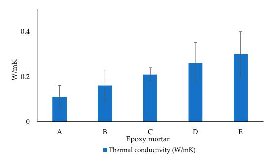
Figure 11. Thermal conductivity (W/mK) of epoxy mortars (A–E) tested after 28 days.
