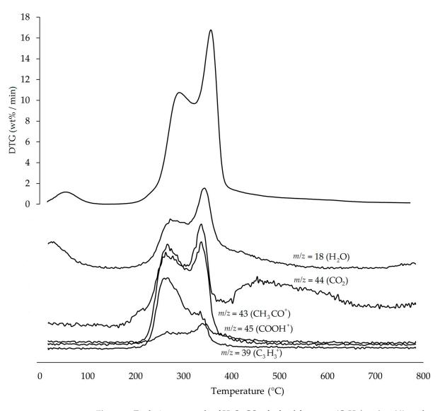
**Figure 5.** Evolutionary trends of H<sub>2</sub>O, CO<sub>2</sub>, furfural fragment (C<sub>3</sub>H<sub>3</sub><sup>+</sup>, m/z = 39), and acetic acid fragments (CH<sub>3</sub>CO<sup>+</sup>, m/z = 43; COOH<sup>+</sup>, m/z = 45) during the heating of the OPP sample. The derivative thermogravimetric (DTG) curve is also displayed for ease of comparison. Intensity of m/z is in arbitrary units.
