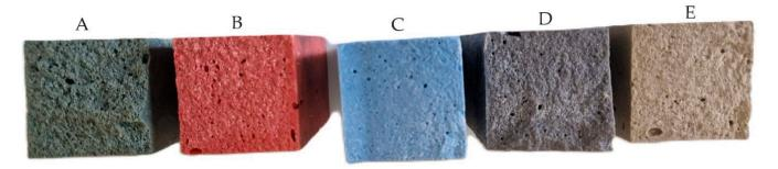
Figure 6. Cross-section of five representative samples of epoxy grout, A-E.
