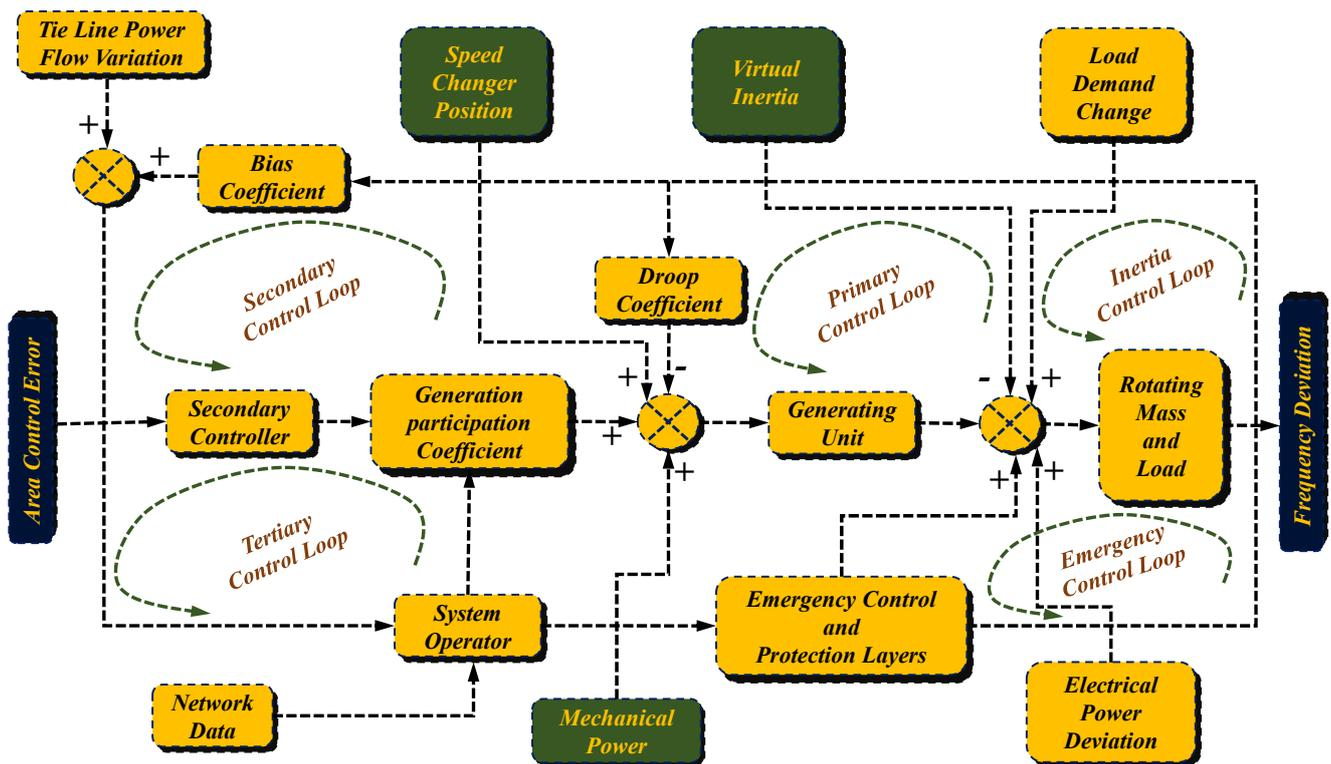
Figure 3. Control frequency in single-area energy system.
