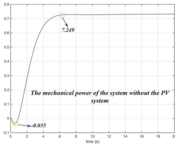
Figure 7. The variations in the mechanical power of the energy network in response to step changes in demand side (without PV system).
