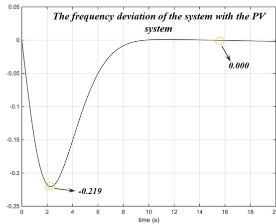
**Figure 9.** The frequency changes within the power grid in response to variations in demand side (with PV system).
