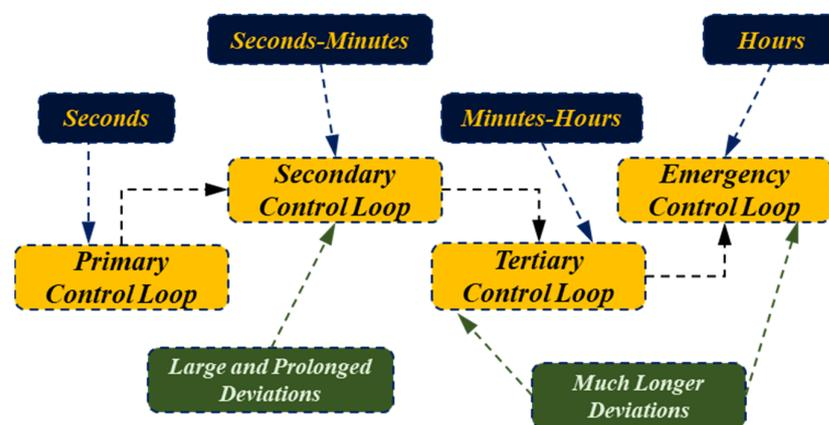
**Figure 1.** Classification and time range of frequency control.
