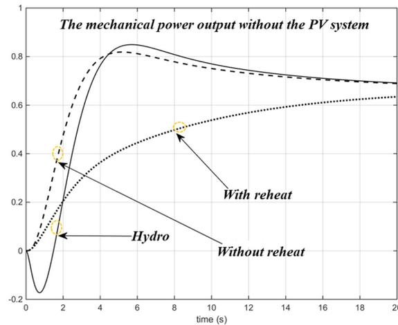
**Figure 8.** The variations in the mechanical power of each power unit within the power system in response to variations in demand side (without PV system).
