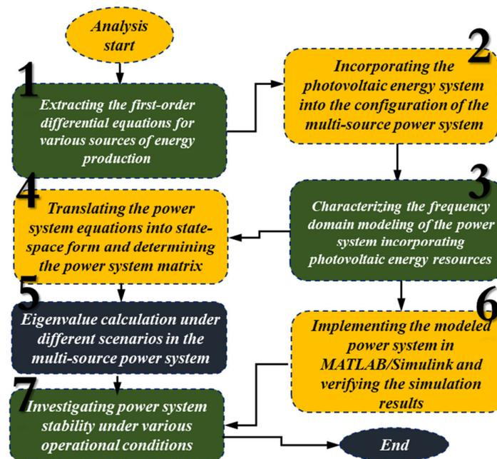
**Figure 5.** The process of simulating the presented power system and investigating the impact of the photovoltaic system.
