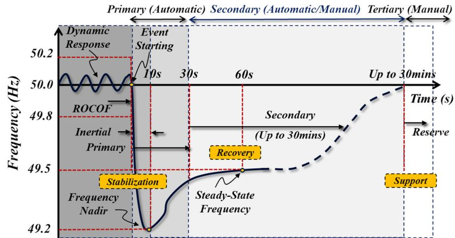
Figure 2. The dynamic reaction of system frequency across various time scales.
