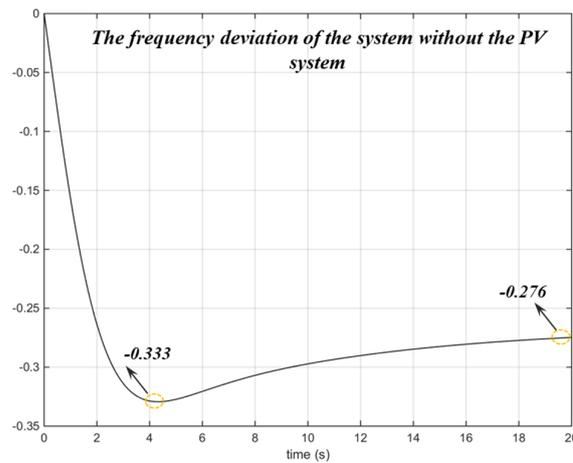
Figure 6. Power system frequency changes for step changes in load demand (without PV system).
