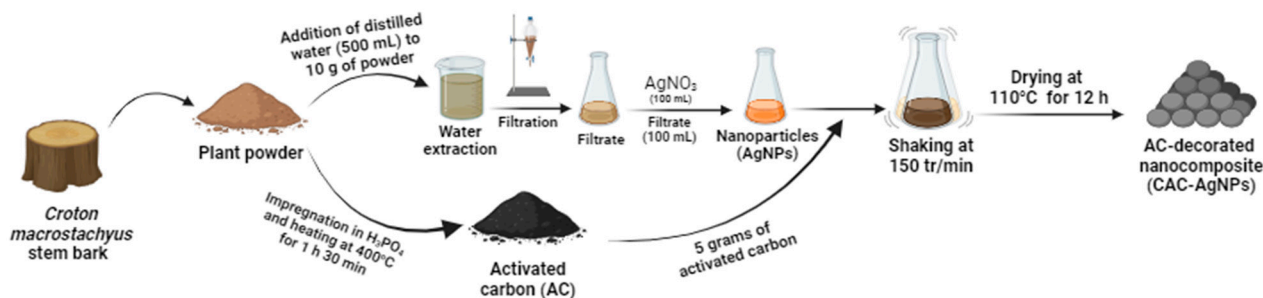
Figure 1. Pictorial representation of the procedure for the green synthesis of silver nanoparticles and nanocomposites from Croton macrostachyus stem bark.
