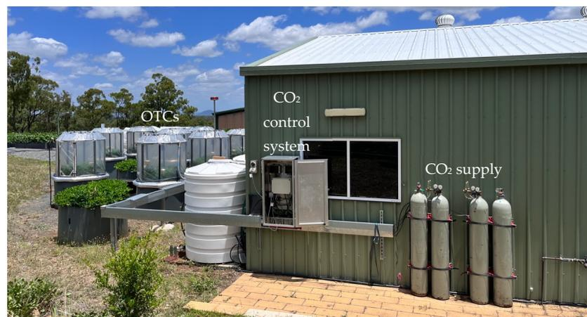
**Figure 2.** Overview of the experimental site, featuring the main components of the facility. The gas cylinders supplying carbon dioxide stand alongside the CO<sub>2</sub> control system, with distinct octagonal-shaped OTCs and control plots without chambers.
