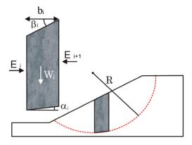
In Bishop's method the factor of safety is determined by trial and errors, using an iterative process, since the factor of safety ( $F_s$ ) appears in both sides of Equation (3).
