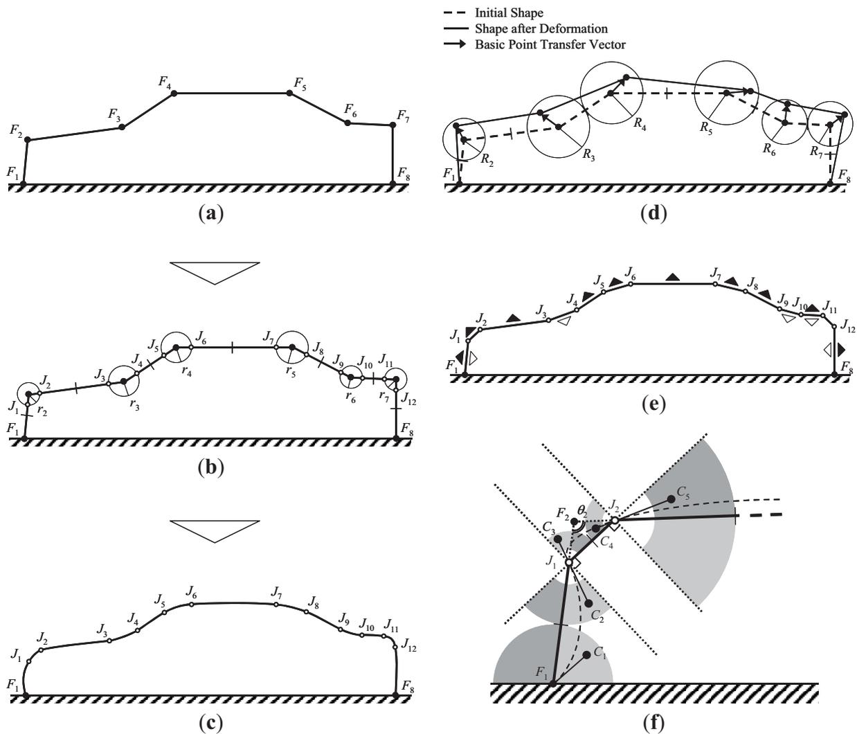
During shape generation, points  $F_1$  and  $F_8$  are fixed, while points  $F_2$  through  $F_7$  are movable. The basic point transfer vector is defined to begin from the basic point toward the deformed points (Figure 15d). The movable ranges of points  $F_2$  through  $F_7$  are defined as circles with radii  $R_2$  through  $R_7$  (Figure 15d). The radii are defined by the following equation:
