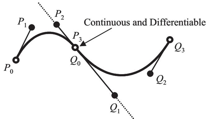
Figure 9 shows a method to express a basic curved profile by a three-dimensional Bézier curve. First, circles with radii  $r_1$  through  $r_7$  are drawn to select the positions of the connection points. The intersection points between the edges of the circles and the polygonal profile  $J_1$  through  $J_{12}$  are assumed to be the connection points. To improve the smoothness of a curved profile, radii  $r_1$  through  $r_7$  are defined as:
