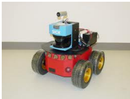
Figure 6. Picture of the mobile robot Pioneer 3AT used in this work. The range sensor laser is mounted on the vehicle.
