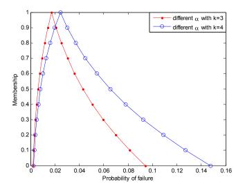
**Figure 9.** Probability of failure for different  $\mu_{\theta}$  values
