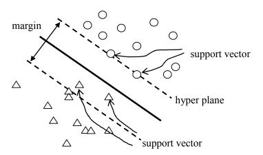
Let  $\{(x_k, y_k), k=1,2,...,N\}$  be the given data sets as the training sample. Each sample data  $x_k \in \mathbb{R}^d$  is distinguished as the *i*-class or *j*-class according to the value of  $y_k$  ( $y_k = \{+1, -1\}$ ). The hyper plane can be formulated as:
