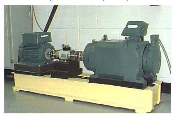
**Figure 2.** Picture of the bearing fault test rig.
