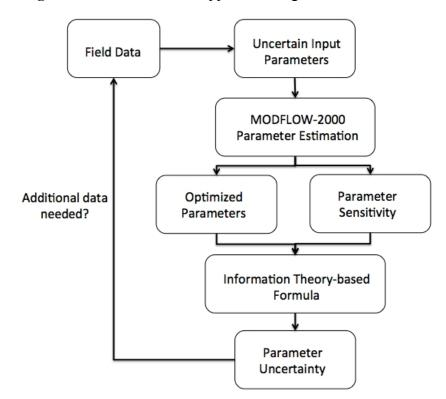
Figure 1. Flowchart of ITb approach using MODFLOW-2000.
