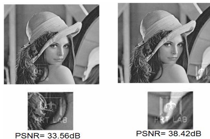
Figure 43. Results for the Lena-Titech logo pair based on the revised watermark embedding circuit for the scheme-designated watermark window on the left and one whose watermark window has been assigned to the extreme lower-right corner by default.
