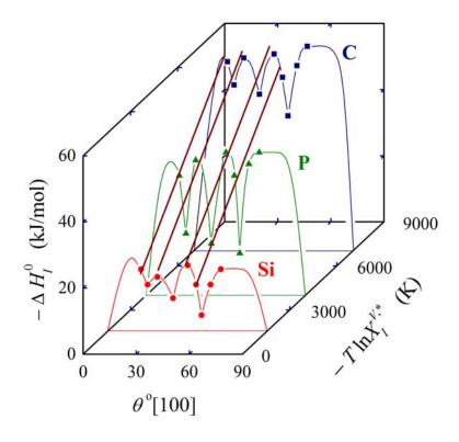
**Figure 6.** Anisotropy of (**a**) the standard enthalpy,  $\Delta H_I^0$ , and (**b**) the standard entropy,  $\Delta S_I^0$ , of Si, P and C segregation for [100] symmetrical grain boundaries in  $\alpha$ -iron [1,4,5].
