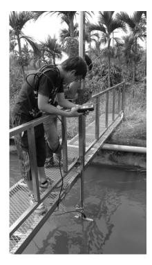
The Wan-Dan Canal is a 3 m wide rectangular channel built with reinforced concrete. To develop a reliable and accurate discharge measurement method for the Wan-Dan Canal, a large amount of data on velocities over the full cross-section is collected. It is conventional to make the nine verticals
