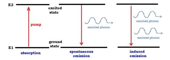
**Figure 1.** Physics: emission and absorption of light quanta.
