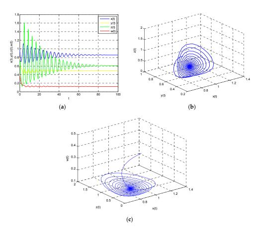
**Figure 11.** The influence of  $\tau_2$  on the stability of Model (22) when  $\tau_1 = 0.1, \tau_2 = 0.05 < \tau_{20} = 0.1429$ : (a) Time-domain plot; (b) energy supply–demand attractor (x(t), y(t), z(t)); and (c) energy supply–demand attractor (x(t), z(t), w(t)).
