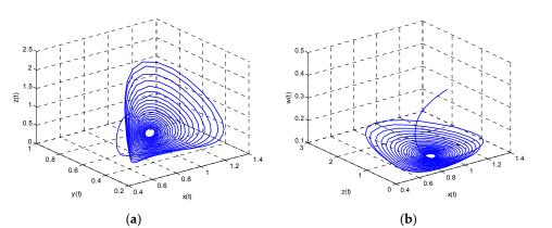
**Figure 5.** The attractor when  $\tau_1 = 0.4 > \tau_{10} = 0.2208$ ,  $\tau_2 = 0$ : (a) x(t), y(t), z(t); and (b) x(t), z(t), w(t).
