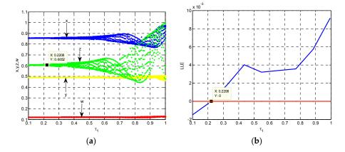
**Figure 1.** The impact of  $\tau_1$  on the stability of Model (22) when  $\tau_2 = 0$ : (**a**) bifurcation diagram; and (**b**) the largest Lyapunov exponent plot.
