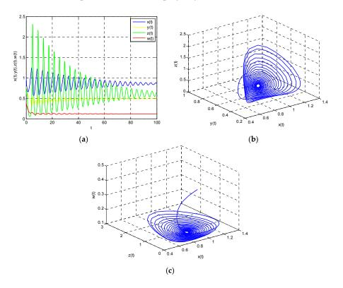
**Figure 18.** Model (23) is unstable when k = 0.6 < 0.7013 for  $\tau_1 = 0.4$ ,  $\tau_2 = 0$ : (a) time-domain plot; (b) energy supply-demand attractor (x(t), y(t), z(t)); and (c) energy supply-demand attractor (x(t), z(t), w(t)).
