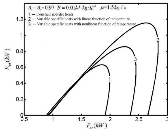
Figure 8. Effects of specific heat models on  $E$  versus  $P$ .
