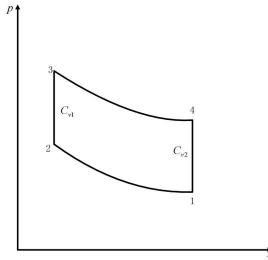
Figure 1.  $p - v$  diagram for the Otto cycle model.
