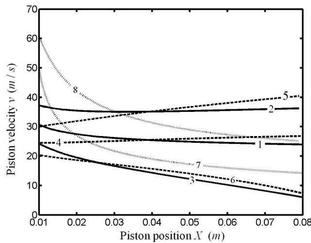
Figure 14. OPM trajectories on the power stroke with different HTAs and OPBs. 1.MEF, Newton's heat transfer law; 2. MEG, Newton's heat transfer law; 3. MW, Newton's heat transfer law; 4. MEF, linear phenomenological heat transfer law; 5. MEG, linear phenomenological heat transfer law; 6. MW, linear phenomenological heat transfer law; 7. MEF, radiative heat transfer law; 8. MEG, radiative heat transfer law.
