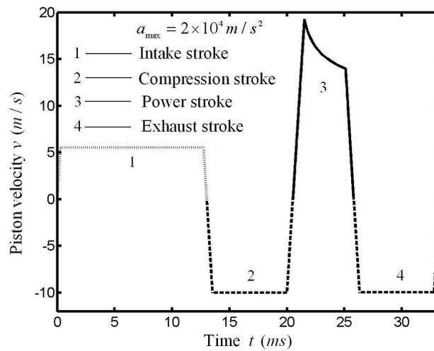
Figure 13. OPM trajectory for MEF of the whole cycle when HTA obeys Newton's HTA.
