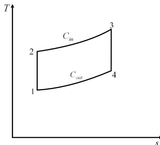
Figure 3.  $T - s$  diagram for the first universal cycle model [101].
