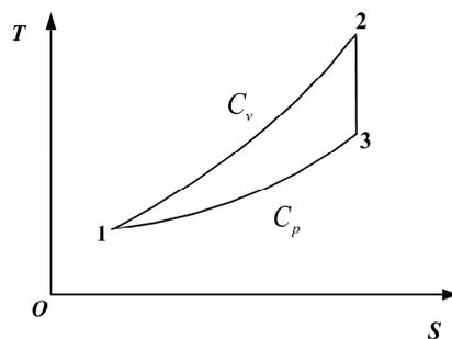
Figure 20.  $T - s$  diagram for the Lenoir cycle model [318,319].
