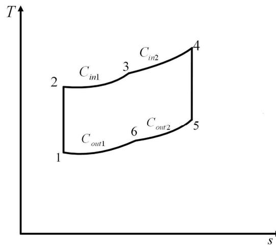
Figure 4.  $T - s$  diagram for the second universal cycle model [72,102].
