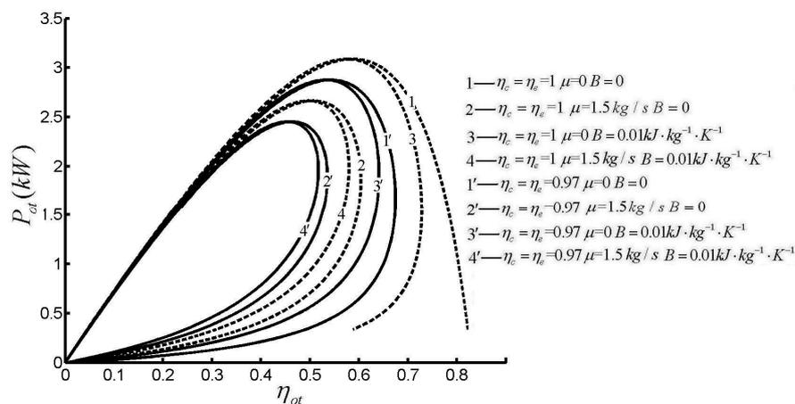
Figure 5. Effects of  $\eta_c$ ,  $\eta_e$ ,  $B$  and  $\mu$  on  $P$  versus  $\eta$ .
