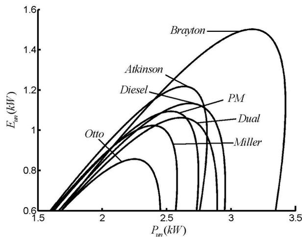
Figure 10. Comparison of  $E$  versus  $P$  of different cycles.
