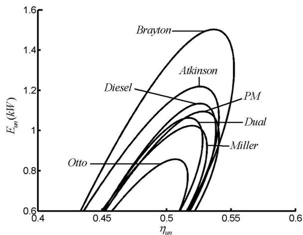
Figure 11. Comparison of  $E$  versus  $\eta$  of different cycles.
