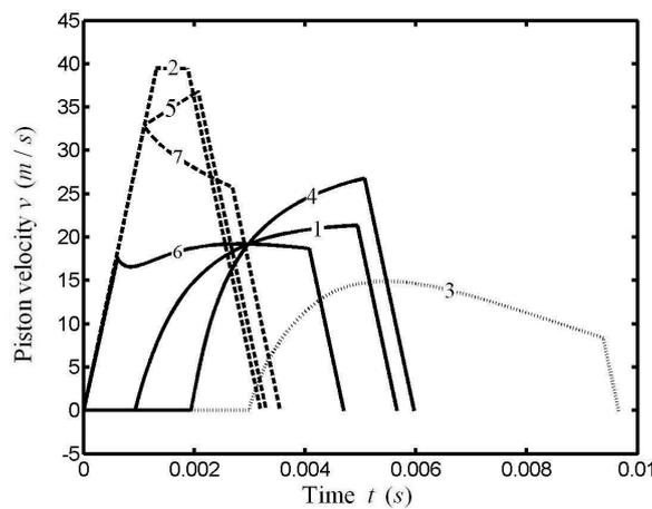
**Figure 15.** Comparison of OPM trajectories with different HTAs and OPBs (velocity). 1. MEF, Newton’s heat transfer law; 2. MEG, Newton’s heat transfer law; 3. MW, Newton’s heat transfer law; 4. MEF, linear phenomenological heat transfer law; 5. MEG, linear phenomenological heat transfer law; 6. MW, linear phenomenological heat transfer law; 7. MEF, radiative heat transfer law; 8. MEG, radiative heat transfer law.
