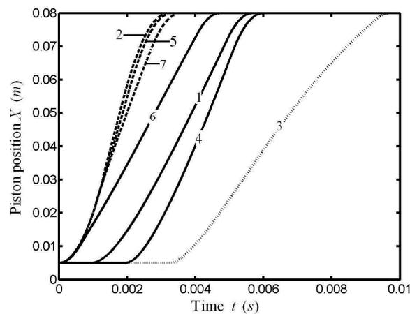
**Figure 17.** Comparison of OPM trajectories with different HTAs and OPBs (displacement). 1. MEF, Newton's heat transfer law; 2. MEG, Newton's heat transfer law; 3. MW, Newton's heat transfer law; 4. MEF, linear phenomenological heat transfer law; 5. MEG, linear phenomenological heat transfer law; 6. MW, linear phenomenological heat transfer law; 7. MEF, radiative heat transfer law; 8. MEG, radiative heat transfer law.
