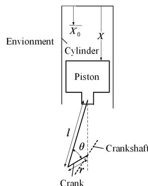
Figure 12. Conventional piston linkage.
