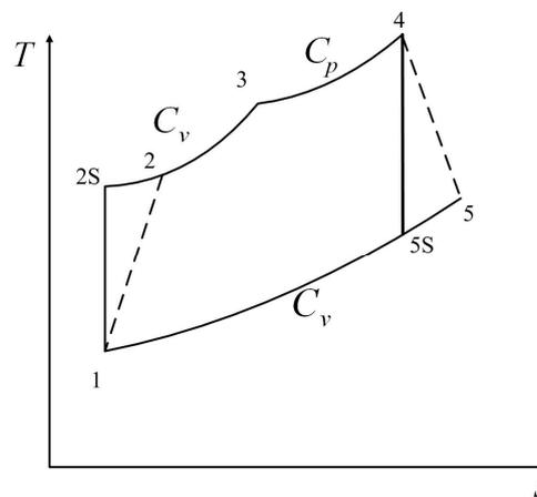
Figure 2.  $T - s$  diagram for the Dual cycle model.
