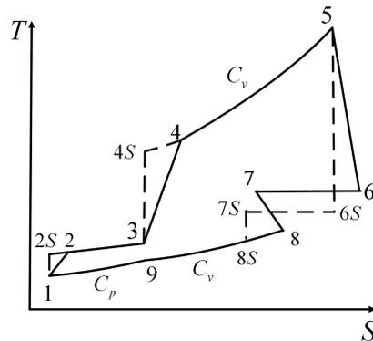
Figure 18.  $T - s$  diagram for irreversible Meletis–Georgiou cycle model [304,309].
