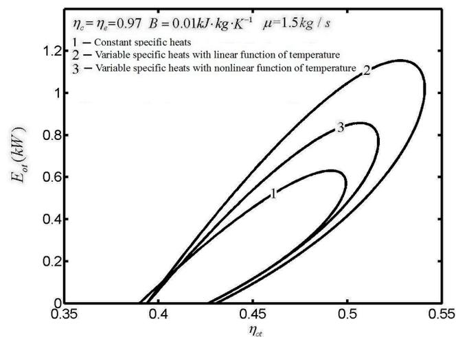
Figure 9. Effects of specific heat models on  $E$  versus  $\eta$ .
