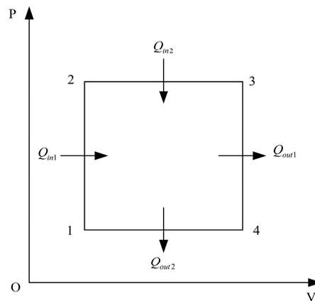
Figure 19.  $p - v$  diagram for the rectangular cycle model [310,311].
