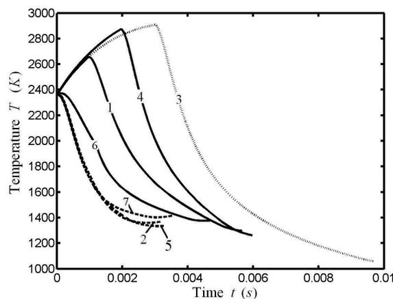
**Figure 16.** Comparison of OPM trajectories with different HTAs and OPBs (temperature). 1. MEF, Newton’s heat transfer law; 2. MEG, Newton’s heat transfer law; 3. MW, Newton’s heat transfer law; 4. MEF, linear phenomenological heat transfer law; 5. MEG, linear phenomenological heat transfer law; 6. MW, linear phenomenological heat transfer law; 7. MEF, radiative heat transfer law; 8. MEG, radiative heat transfer law.
