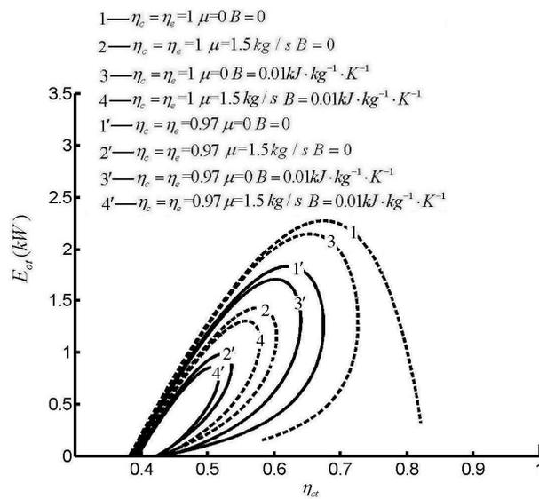
Figure 7. Effects of  $\eta_c$ ,  $\eta_e$ ,  $B$  and  $\mu$  on  $E$  versus  $\eta$ .
