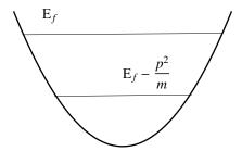
**Figure 3.** The effective Fermi level in k is shifted downward by  $p^2/2m$ .
