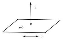
**Figure 2.** Flat boundary surface and the "tangential" and "longitudinal" wave-vectors *p* and *k*.
