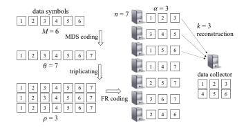
**Figure 1.** Structure of a [(7,6), 3, (7,3,3)] distributed replication-based exact simple storage (DRESS) code.
