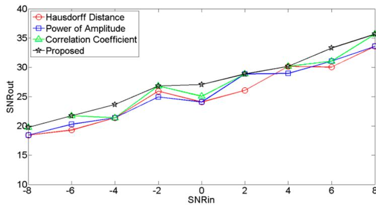
Figure 9. SNR<sub>in</sub> vs. SNR<sub>out</sub> of signal contaminated by factory noise.
