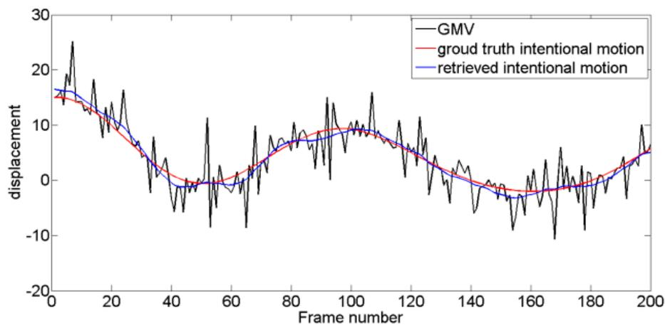
Figure 18. Resulting intentional motion compared with the ground truth in Test 4 video sequence.
