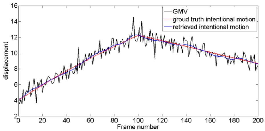
Figure 15. Resulting intentional motion compared with the ground truth in Test 1 video sequence.
