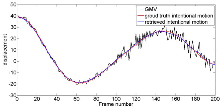
Figure 17. Resulting intentional motion compared with the ground truth in Test 3 video sequence.
