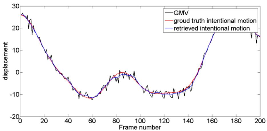
Figure 16. Resulting intentional motion compared with the ground truth in Test 2 video sequence.
