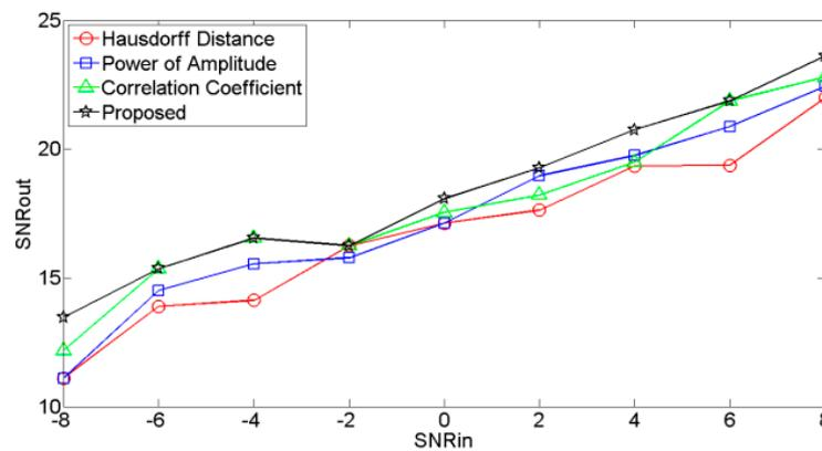
Figure 7. SNRin vs. SNRout of signal contaminated by Gaussian noise.
