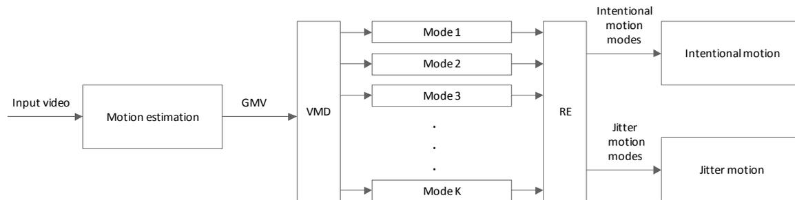
**Figure 1.** Proposed DIS framework based on VMD and RE.
