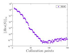
**Figure 4.** Effects of the number of collocation points number on the residual error of the solute concentration profile  $||Res(S)||_{\infty}$  when n = 3, A = 0.3, Pr = 7, Ha = 0.5, Nr = 0.2, Nb = 0.5, Nt = 0.5, Nd = 0.02, Ld = 0.02, Sc = 7,  $R_0 = 0.3$ , Bi = 0.2.
