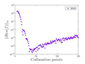
**Figure 2.** Effects of the number of collocation points number on the residual error of the velocity profile  $||Res(f)||_{\infty}$  when n = 3, A = 0.3, Pr = 7, Ha = 0.5, Nr = 0.2, Nb = 0.5, Nt = 0.5, Nd = 0.02, Ld = 0.02, Sc = 7,  $R_0 = 0.3$ , Bi = 0.2.
