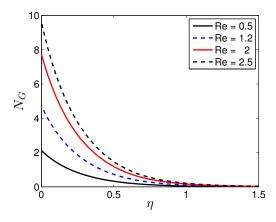
**Figure 23.** Effects of the Reynolds number *Re* on the entropy generation number  $N_G$  when Nr = 0.2, Br = 1,  $\Omega = 1$ , Ha = 0.5 and  $\Sigma = 0.5$ .
