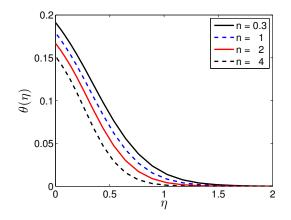
**Figure 7.** Effects of the stretching parameter *n* on  $\theta(\eta)$  where A = 0.3, Ha = 0.5, Nr = 0.2, Pr = 10, Nb = 0.5, Nt = 0.5, Nd = 0.02, Sc = 7,  $R_0 = 0.3$ , Ld = 0.02, Bi = 0.2.
