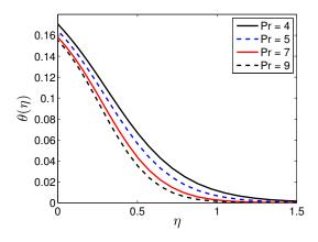
**Figure 14.** Effects of the Prandtl number (*Pr*) on  $\theta(\eta)$  for  $n = 3, A = 0.3, Ha = 0.5, Nr = 0.2, Nb = 0.5, Nt = 0.5, Nd = 0.02, Sc = 7, R_0 = 0.3, Ld = 0.02, \beta_i = 0.2.$
