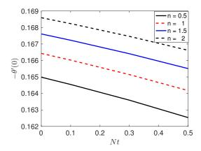
**Figure 29.** Effect of the thermophoresis number (*Nt*) and the stretching sheet parameter (*n*) on the Nusselt number  $(-\theta'(0))$  when A = 0.3, Ha = 0.5, Pr = 7, Nr = 0.2, Nb = 0.5, Nd = 0.02, Ld = 0.02, Sc = 7,  $R_0 = 0.3$ , Bi = 0.2.
