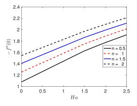
**Figure 28.** Effect of the magnetic field *Ha* and the stretching sheet parameter *n* on the skin friction -f''(0) when A = 0.3, Pr = 7, Nr = 0.2, Nb = 0.5, Nt = 0.5, Nd = 0.02, Ld = 0.02, Sc = 7,  $R_0 = 0.3$ , Bi = 0.2.
