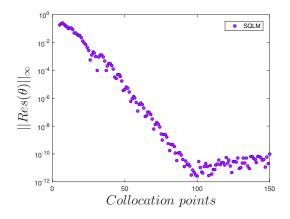
**Figure 3.** Effects of the number of collocation points number on the residual error of the temperature profile  $||Res(\theta)||_{\infty}$  when n = 3, A = 0.3, Pr = 7, Ha = 0.5, Nr = 0.2, Nb = 0.5, Nt = 0.5, Nd = 0.02, Ld = 0.02, Sc = 7,  $R_0 = 0.3$ , Bi = 0.2.
