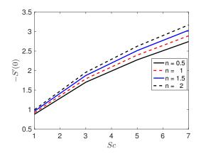
**Figure 30.** Effect of the Schmidt number *Sc* and the stretching sheet parameter *n* on the Sherwood number -S'(0) when A = 0.3, Ha = 0.5, Pr = 7, Nr = 0.2, Nb = 0.5, Nd = 0.02, Ld = 0.02, Nt = 0.5,  $R_0 = 0.3$ , Bi = 0.2.
