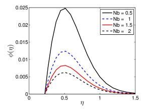
**Figure 21.** Effects of the Brownian motion parameter (*Nb*) on  $\phi(\eta)$  when  $n = 3, A = 0.3, Ha = 0.5, Nr = 0.2, Pr = 7, Nt = 0.5, Nd = 0.02, Sc = 7, R_0 = 0.3, Ld = 0.02, Bi = 0.2.$
