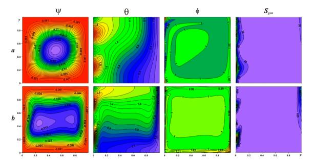
**Figure 5.** Streamlines  $\psi$ , isotherms  $\theta$ , nanoparticles volume fraction  $\phi$  and total entropy generation  $S_{gen}$  for  $\varepsilon = 1.0$ ,  $\kappa = 2.0$ : (a)  $Ra = 10^3$ , (b)  $Ra = 10^5$ .
