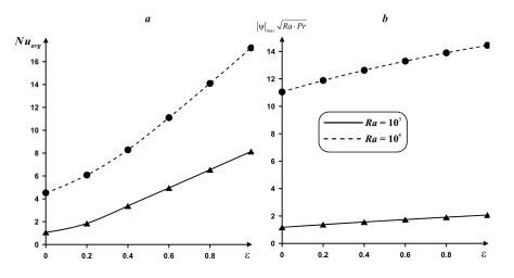
**Figure 9.** Variations of average Nusselt number (**a**) and fluid flow rate (**b**) for  $\kappa$  = 2.0 and different values of amplitude  $\varepsilon$  and Rayleigh number.
