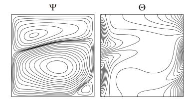
**Figure 4.** Obtained streamlines  $\Psi$  and isotherms  $\Theta$  at  $Ra = 10^5$  and phase deviation  $\varphi = \pi/2$ .
