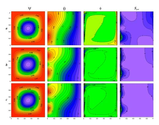
**Figure 7.** Streamlines  $\psi$ , isotherms  $\theta$ , nanoparticles volume fraction  $\phi$  and total entropy generation  $S_{gen}$  for  $Ra = 10^3$ ,  $\kappa = 2.0$ : (a)  $\varepsilon = 0.2$ , (b)  $\varepsilon = 0.6$ , (c)  $\varepsilon = 0.8$ .
