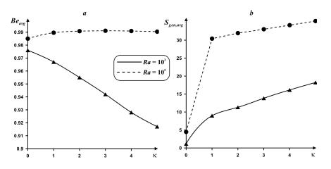
**Figure 14.** Variations of average Bejan number (**a**) and average entropy generation (**b**) for  $\varepsilon$  = 1.0 and different values of wavy number and Rayleigh number.
