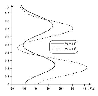
**Figure 6.** Profiles of local Nusselt number along left vertical wall for  $\varepsilon = 1.0$ ,  $\kappa = 2.0$  and different Rayleigh numbers.
