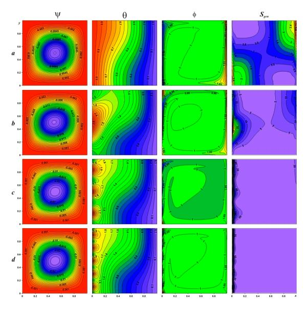
**Figure 11.** Streamlines  $\psi$ , isotherms  $\theta$ , nanoparticles volume fraction  $\phi$  and total entropy generation  $S_{gen}$  for  $Ra = 10^3$ ,  $\varepsilon = 1.0$ : (**a**)  $\kappa = 0.0$ , (**b**)  $\kappa = 1.0$ , (**c**)  $\kappa = 3.0$ , (**d**)  $\kappa = 5.0$ .
