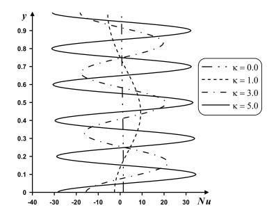
**Figure 12.** Profiles of local Nusselt number along left vertical wall for  $Ra = 10^3$ ,  $\varepsilon = 1.0$  and different values of wave number.
