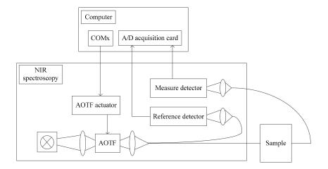
Figure 5. The diagram of measure system structure.
