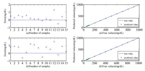
Figure 9. The errors and the predicted values of two methods (a) SVR model (b) PLSR model.
