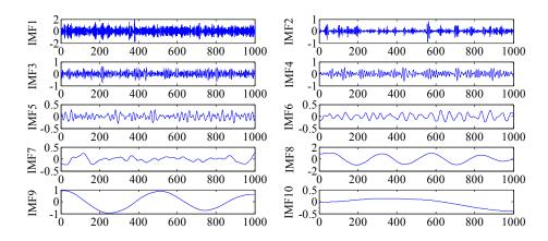
**Figure 2.** The IMF obtained by improved CEEMDAN algorithm.
