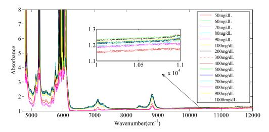
Figure 6. The near-infrared spectral data of glucose solution.
