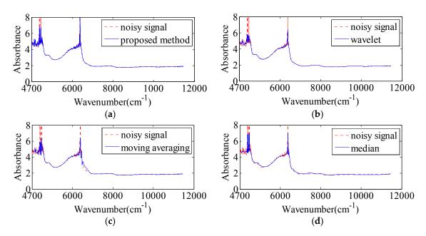
**Figure 7.** The reconstructed results of four methods (700 mg/dL). (a) Proposed method; (b) Wavelet; (c) Moving averaging; (d) Median.
