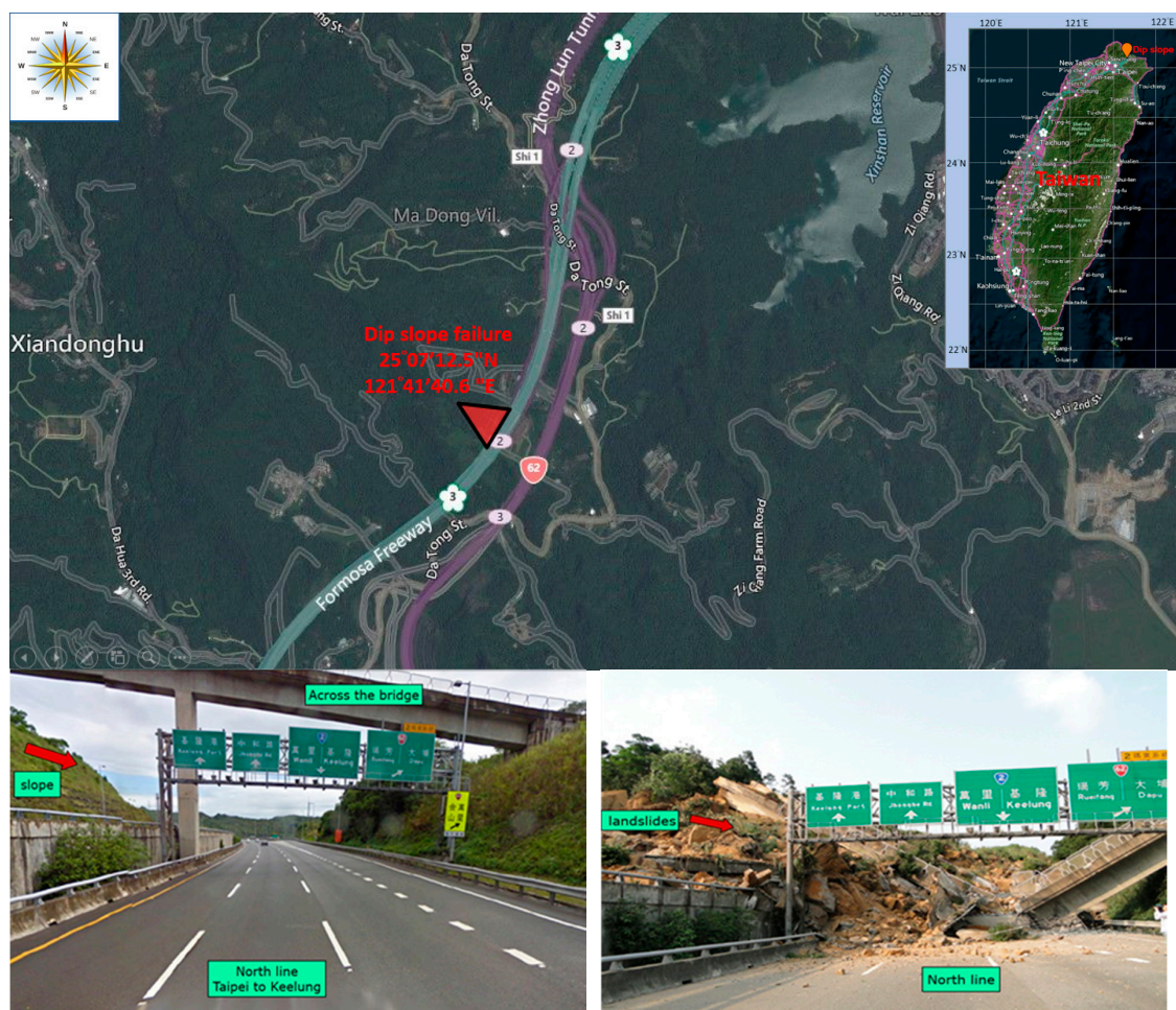
Figure 1. Large-scale landslides on a dip slope on the Taiwan Formosan Freeway.
