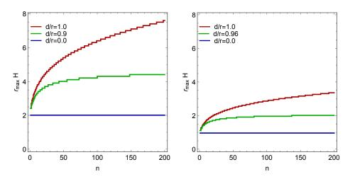
**Figure 4.**  $r_{\text{max}}$  as a function of number of detectors *n*. Left panel: the massless conformal scalar field with  $\theta = \pi/2$ . Right panel: the massless minimal scalar field with  $\theta = \pi/4$ , N = 10. For both types of scalar fields, with d/r = 1,  $r_{\text{max}}$  exceeds the horizon scale 2 H<sup>-1</sup> as the number of detectors increases.
