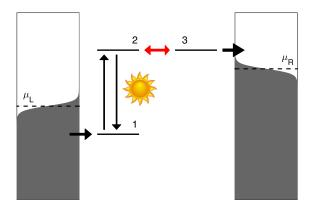
Figure 1. Sketch of the molecular donor-bridge-acceptor (DBA) heat engine model.
