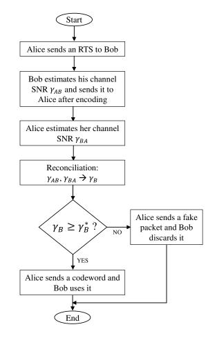
Figure 3. Flow chart of the transmission of a packet according to the OOT-FP protocol.
