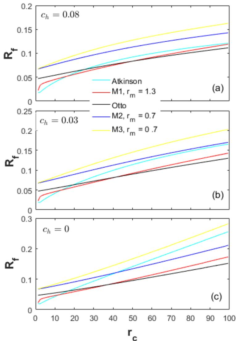
Figure 9. Ratios of friction loss for different heat-transfer weights.
