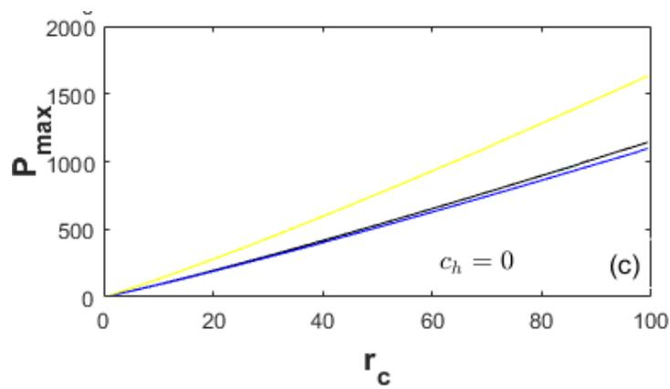
Figure 6. Peak cylinder pressure for different heat-transfer weights.
