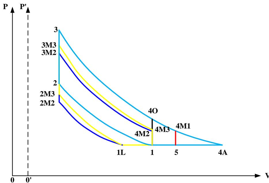
Figure 1. P-V diagrams for the Otto, Atkinson and Miller cycles.
