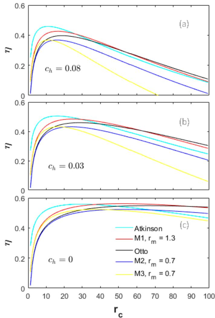
Figure 3. Energy efficiency at different heat-transfer weights.
