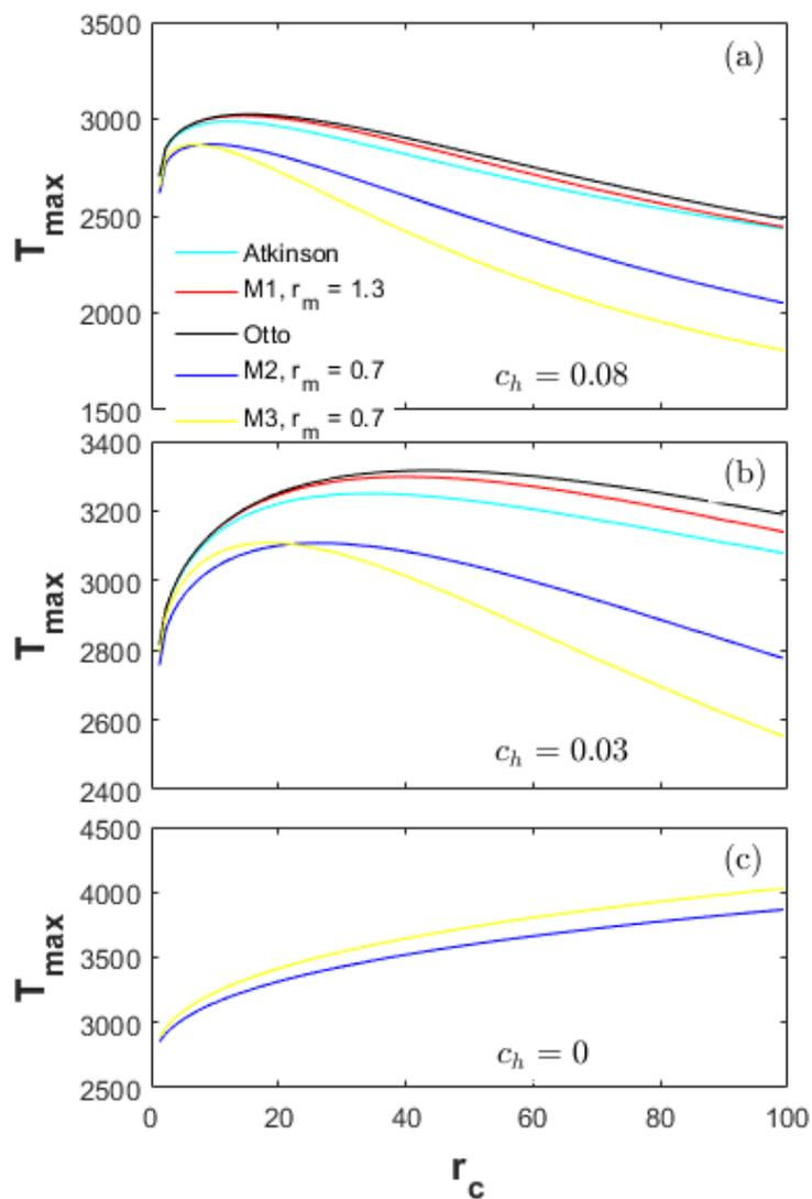
Figure 7. Peak in-cylinder gas temperature for different heat-transfer weights.
