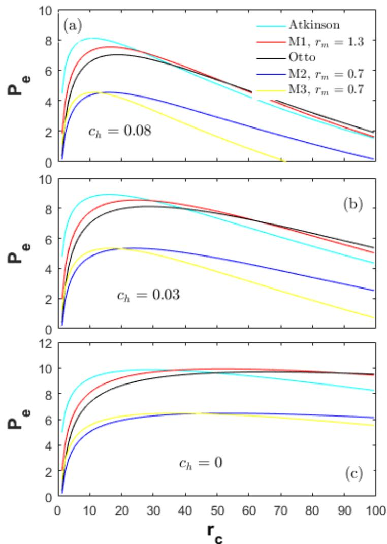
Figure 2. Effective power at different heat-transfer weights.
