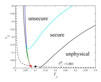
**Figure 8.** Secure and unsecure regions of the UD protocol under realistic detection condition. The parameters are set to  $\beta = 0.99$ ,  $V_M = 3$ ,  $T_x = 0.1$ ,  $\varepsilon_x = 0.01$ ,  $\eta = 0.6$ , and  $v_{el} = 0.1$ .
