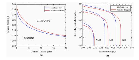
**Figure 3.** (a) Secure and unsecure regions of the SY protocol using ideal homodyne detector ( $\eta = 1, v_{el} = 0$ ) and realistic homodyne detector ( $\eta = 0.6, v_{el} = 0.1$ ); (b) Secret key rate versus the excess noise for different channel losses.
