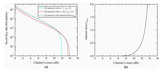
**Figure 10.** (a) Minimum secret key rate as a function of the channel losses; (b) Optimal choice of  $\chi_{\text{hom}}$  that maximizes the secret key rate in (a). The other parameters are  $\beta = 0.99$ ,  $\varepsilon_x = 0.04$ ,  $V_M = 3$ , and  $V_{\nu}^{B_1} \approx 1 + T_x \varepsilon_x$ .
