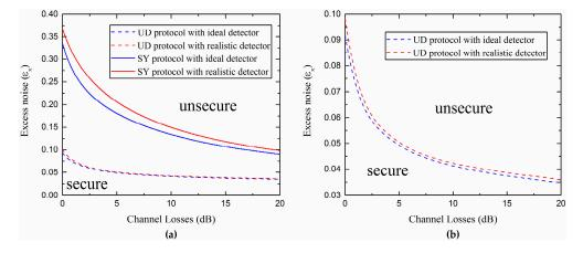
**Figure 9.** (a) Comparison between secure and unsecure regions for the SY coherent-state protocol and UD coherent-state protocol under different detection conditions; (b) Secure and unsecure regions of the UD protocol using an ideal homodyne detector ( $\eta = 1, v_{el} = 0$ ) and a realistic one ( $\eta = 0.6, v_{el} = 0.1$ ). Here we consider  $V_M = 3, \beta = 0.99$ , and the estimated value  $V_y^{B_1} \approx 1 + T_x \varepsilon_x$ .
