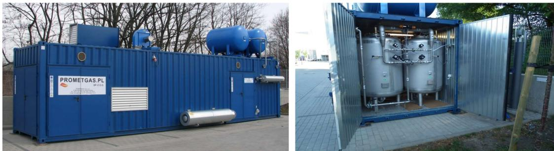
**Figure 5.** Mobile pilot installation Vacuum-Pressure Swing Adsorption (VPSA-O<sub>2</sub>) for extracting oxygen from the air.
