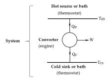
Figure 1. Schematic representation of the thermo-mechanical engine.
