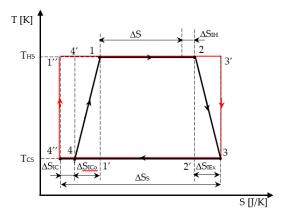
**Figure 2.** Representation of the Carnot engine cycle with internal irreversibility and the corresponding reversible one (in red) in T-S diagram.
