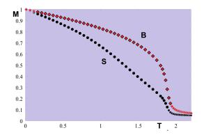
**Figure 24.** Surface magnetization S (circles) and 2nd-layer magnetization B (diamonds) versus *T* in unit of  $J/k_B$  for the non-frustrated case  $J_s = 0.5$  with  $I = I_s = 0.1$ , L = 36.
