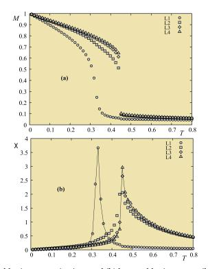
**Figure 28.** (a) Layer sublattice magnetizations and (b) layer sublattice susceptibilities of first two cells vs. *T* for  $J_s = -0.5$ , D = 0.1 (J = -1).  $L_1$  to  $L_4$  indicate data for layer 1 to 4. The susceptibility of layer 1 is divided by a factor 5 for presentation scale convenience.
