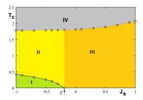
**Figure 26.** Monte Carlo results of the phase diagram in the space ( $J_s$ , T) for the classical Heisenberg model with  $N_z = 4$ ,  $I = |I_s| = 0.1$ . Phases I to IV are defined in Figure 23.
