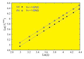
**Figure 35.**  $\ln V_1^{\text{max}}$  versus *L* in the  $\ln - \ln$  scale for  $N_z = 11$  (**a**) without PBC in *z* direction (**b**) with PBC in *z* direction. The slope values are given on the plot.
