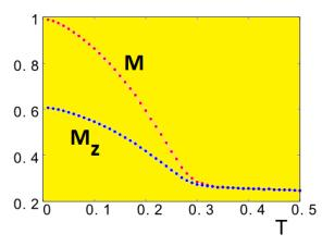
**Figure 39.** Order parameter *M* (red symbols) defined in Equation (77) versus *T*, for H = 0.5 and lattice size 1800 × 1800. The projection  $M_z$  versus *T* (blue symbols) of  $S_z$  on  $S_0^z$  of the GS as defined in Equation (77) but for the *z* components only.
