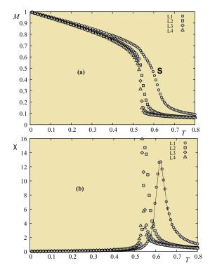
**Figure 30.** (a) Layer sublattice magnetizations and (b) layer sublattice susceptibilities of first two cells vs. *T* for  $J_s = -1$  with D = 0.1 (J = -1).  $L_1$  to  $L_4$  indicate data for layer 1 to 4.
