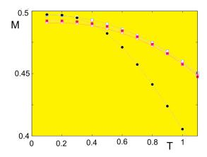
**Figure 33.** Layer magnetizations versus *T* for  $J_2/J_1 = -1.4$  with d = 0.1,  $N_z = 8$ . Black circles, blue void squares, magenta squares, and red void circles are for first, second, third, and fourth layers, respectively. Magnetization crossovers at low *T* are seen. See text for explanation.
