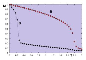
**Figure 25.** Surface magnetization S (circles) and 2nd-layer magnetization B (diamonds) versus *T* in unit of  $J/k_B$  for the frustrated case  $J_s = -0.5$  with  $I = -I_s = 0.1$ , L = 36.
