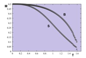
**Figure 22.** Surface (*S*) and 2nd-layer (*B*) magnetizations versus *T* for the non-frustrated case where  $J_s = 0.5$  with  $I = I_s = 0.1$ .
