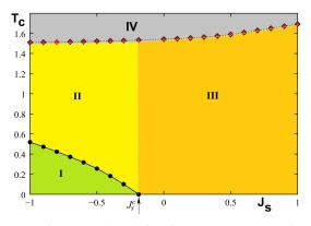
**Figure 23.** Phase diagram in the space ( $J_s$ , T) for the quantum Heisenberg model with  $N_z = 4$ ,  $I = |I_s| = 0.1$ . Phase I is the surface non-collinear phase, phase II has surface disorder and bulk order, phase III and IV are ferromagnetic and paramagnetic phases, respectively.
