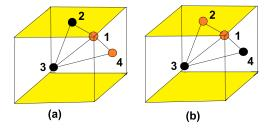
**Figure 27.** Ground-state spin configuration of the surface fcc cell: (a) type I for  $J_s < -0.5$ ; (b) type II for  $J_s > -0.5$  (J = -1). Black and red circles indicate up and down spins, respectively. The vertical axis is the *z* axis. The *x* and *y* axes along the cube in the yellow plane form with the *z* axis a direct triad.
