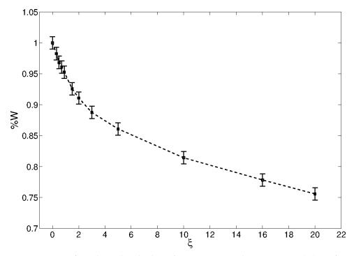
**Figure 5.** Percentage of exactly predicted values of memristors according to Equation (13) as a function of  $\xi$ . The error bar are calculate from 100 samples, with approximately 800 memristors (on average) and  $\xi = 10$ ,  $\alpha = 0.1$  and  $\beta = 1$ , with the vector S drawn at random between [-0.5, 5].
