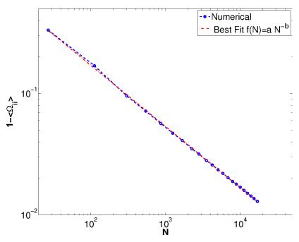
**Figure 4.** Scaling of the components  $\Omega_{ii}$  as a function of the number of memristors for randomly generated circuits.
