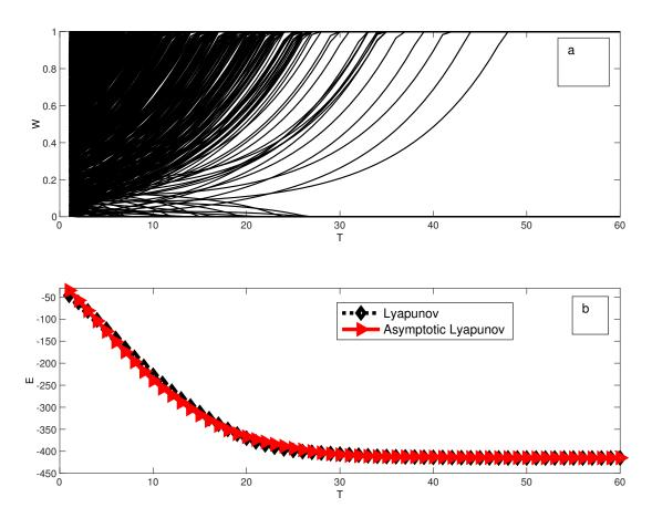
**Figure 1.** Dynamics of the memory is shown in Figure (a) and the corresponding evolution of the Lyapunov function of Equation (A1) ((b), continuous line) for 8750 memristors and for the asymptotic function of Equation (6) Figure ((b)-dashed line). We considered  $\alpha=0.1$ ,  $\beta=1$  and  $\xi=10$ , for  $\Omega_{ij}$  from a random circuit of the Erdos-Renyi type with p=0.9. The sources  $\vec{S}$ 's elements were chosen at random between [-0.05, 0.05].
