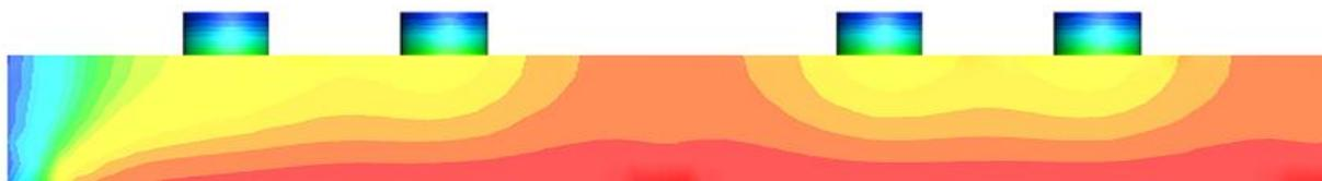
**Figure 5.** Local magnification of inlet water vapor concentration distribution in Model B under static wind conditions.
